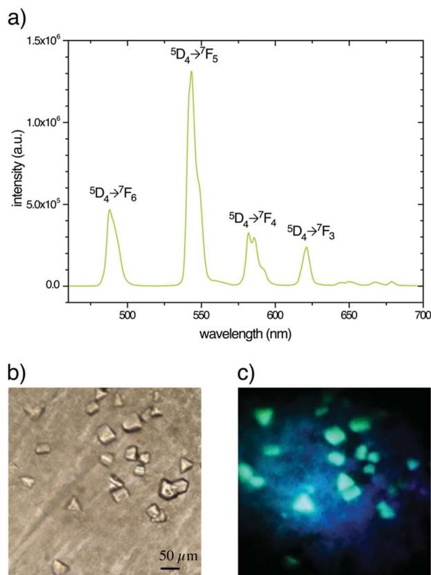
Fig. 7 (a) Luminescence spectrum of Tb-Xo4 in aqueous solution ( $\lambda_{\text{ex}} = 290$  nm). MDH crystals obtained with 10 mM of the complex observed (b) in transmission mode and (c) under UV light irradiation (365 nm).
