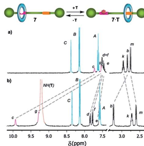
Fig. 4 Selected regions of the  $^1\text{H}$  NMR spectra (400 MHz,  $\text{CD}_2\text{Cl}_2$ , 298 K) of (a) shuttle 7 and (b) after adding an excess (20 equiv.) of *N*-hexylthymine (T) (see Scheme 2 for signal assignments).
