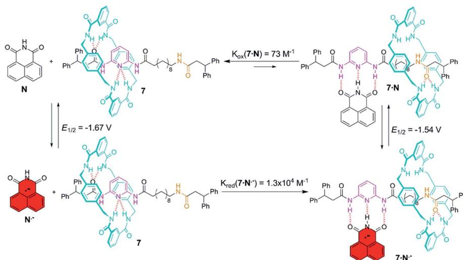
Fig. 6 Anion radical-driven ring shuttling in the two-station [2]rotaxane 7.
