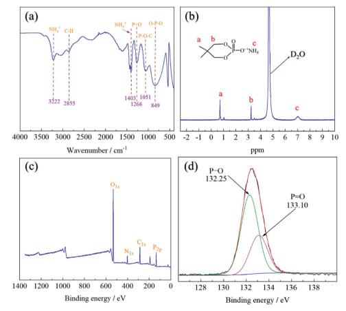
Fig. 3 FT-IR spectrum (a), <sup>1</sup>H-NMR spectrum (b), total XPS spectra (c) and high-resolution P<sub>2p</sub> spectra (d) of PNPG.
