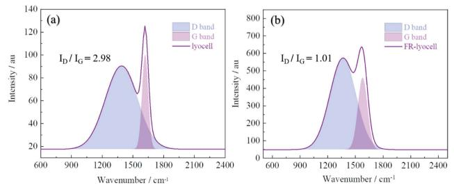
Fig. 11 Raman spectra of the char residue of lyocell fibers (a) and FR-lyocell (b).
