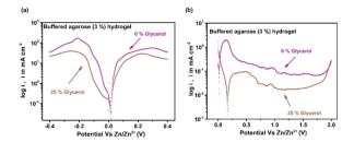
Fig. 5 (a) Stability of Zn metal and (b) carbon coated Ni current collector in the buffered 3% agarose hydrogel electrolyte containing 1 M Zn<sup>2+</sup> without glycerol and in the presence of 25% glycerol (replacing the water in the hydrogel).
