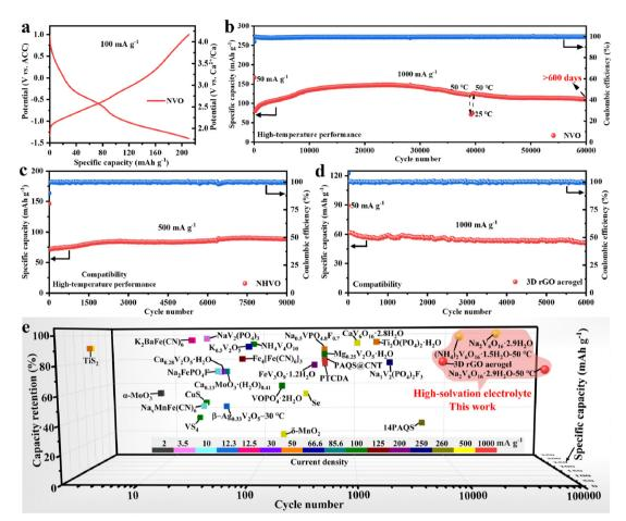
Fig. 4 High-temperature performance and compatibility of high-solvation electrolytes. (a) Galvanostatic charge/discharge profiles of NVO at 100 mA  $g^{-1}$  and 50 °C. (b)-(d) Cycling performances of (b) NVO at 1000 mA  $g^{-1}$  and 50 °C, (c) NHVO at 500 mA  $g^{-1}$  and 50 °C and (d) 3D rGO aerogel at 1000 mA  $g^{-1}$ . (e) Comparison of the  $Ca^{2+}$  storage performance of the 3D rGO aerogel, NHVO, and NVO with reported cathode materials for CIBs in organic electrolyte. 20-45
