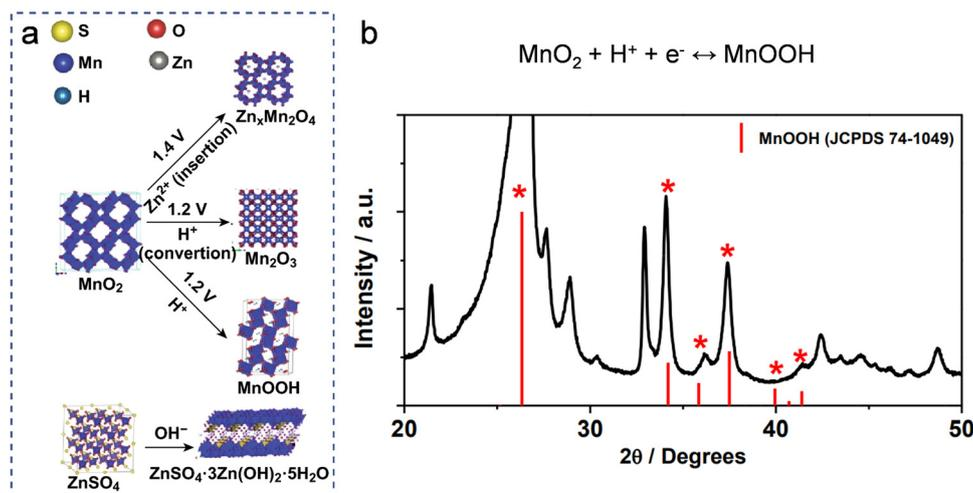
Fig. 8 Conversion mechanism based on protonation/deprotonation. (a) Schematic diagram of phase evolution during discharge. Reproduced with permission from ref. 124. Copyright 2019 Springer Science & Business Media. (b) The XRD pattern of  $\alpha\text{-MnO}_2$  in its fully discharged state unequivocally validates the generation of  $\text{MnOOH}$ . Reproduced with permission from ref. 125. Copyright 2016 Springer Science & Business Media.
