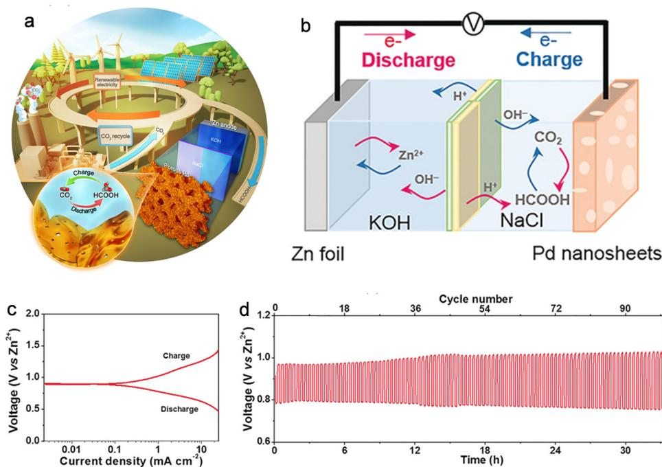
Fig. 27 Zn–CO<sub>2</sub> batteries. (a) Illustration outlining the prospective application of the Zn–CO<sub>2</sub> battery in future energy storage. (b) Visual representation elucidating the operational principles of a reversible aqueous Zn–CO<sub>2</sub> battery. (c) Charge and discharge polarization curve. (d) Charge and discharge cycle curve under 0.56 mA cm<sup>-2</sup> constant current. Reproduced with permission from ref. 179. Copyright 2018 John Wiley & Sons.
