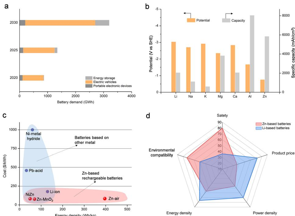
**Fig. 1** Motivation to study Zn-based batteries. (a) Projected battery demand (GWh) for portable electronic devices, electric vehicles, and energy storage systems spanning the period 2020 to 2030. (b) Redox potential and specific capacity of various metals. (c) Energy density and price of various batteries. (d) Comparison of Zn-based batteries and Li-based batteries from multiple metrics.
