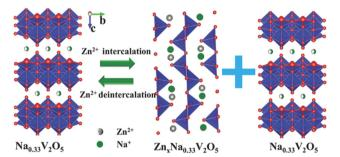
Fig. 4 Schematic depiction of the Zn<sup>2+</sup> insertion mechanism in the Na<sub>0.33</sub>V<sub>2</sub>O<sub>5</sub> cathode. Reproduced with permission from ref. 108. Copyright 2018 John Wiley & Sons.
