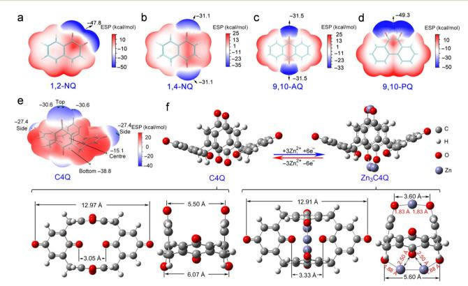
Fig. 10 Inferring the active site and structural evolution of guinone cathodes. (a)-(e) The ESP-mapped van der Waals surface of diverse organic molecules. (f) Optimized molecular structure of C4Q before and after Zn<sup>2+</sup> absorption. Reproduced with permission from ref. 147. Copyright 2018 American Association for the Advancement of Science.
