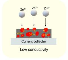
Fig. 14 Schematic diagram of the adverse effects of various factors (strong repulsive effect, insufficient active sites, and low conductivity) on the theoretical capacity of cathode materials.
