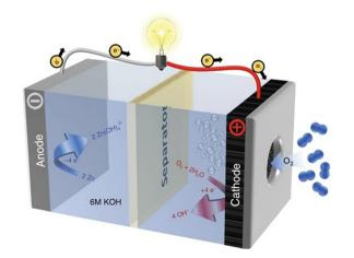
Fig. 11 Illustration depicting the fundamental structure and reaction mechanism of Zn-air batteries. Reproduced with permission from ref. 155. Copyright 2020 Springer Science  $\theta$  Business Media.
