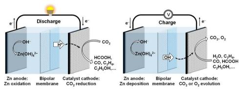
Fig. 12 Illustration depicting the discharge and charging processes of an aqueous Zn-CO<sub>2</sub> battery. Reproduced with permission from ref. 166. Copyright 2022 John Wiley & Sons.
