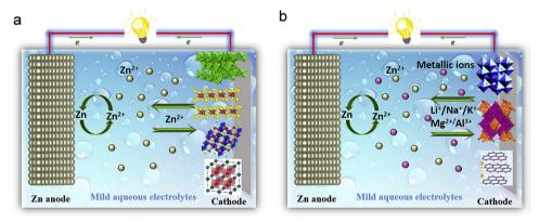
Fig. 7 Comparing the operational principles of Zn-ion batteries. (a) Zn-ion battery (Zn<sup>2+</sup> insertion/extraction mechanism). (b) Hybrid Zn-ion battery (Li/ Na/K/Mg/Al insertion/extraction mechanism). Reproduced with permission from ref. 114. Copyright 2019 Elsevier.
