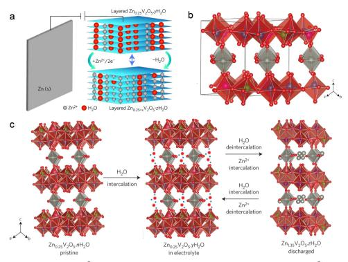
Fig. 6 Co-insertion mechanism of H<sub>2</sub>O and Zn<sup>2+</sup>. (a) Schematic representation illustrating the co-insertion of H<sub>2</sub>O and Zn<sup>2+</sup> during discharge. (b) Crystal structure depiction of  $Zn_{0.25}V_2O_5$ . (c) Schematic diagram delineating the reversible co-insertion/extraction process of  $H_2O$  and Zn ions in  $Zn_{0.25}V_2O_5$ . nH<sub>2</sub>O. Reproduced with permission from ref. 112. Copyright 2016 Springer Science & Business Media.
