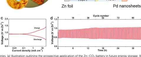
Fig. 27 Zn-CO<sub>2</sub> batteries. (a) Illustration outlining the prospective application of the Zn-CO<sub>2</sub> battery in future energy storage. (b) Visual representation elucidating the operational principles of a reversible aqueous Zn-CO<sub>2</sub> battery. (c) Charge and discharge polarization curve. (d) Charge and discharge cycle curve under 0.56 mA cm<sup>-2</sup> constant current. Reproduced with permission from ref. 179. Copyright 2018 John Wiley & Sons.
