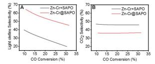
Fig. 2 Relationship curves of CO conversion vs. (A) light olefin selectivity and (B)  $CO_2$  selectivity of physical mixture and capsule catalysts. Reaction conditions:  $H_2/CO = 2.0$ , P = 2.0 MPa, T = 400 °C.
