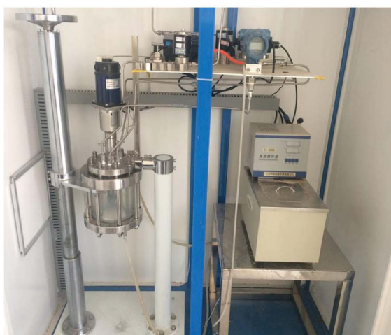
Fig. 1 Physical and schematic diagram of the experimental setup ((1) positive pressure pump, (2) vacuum pump, (3) flowmeter, (4) circulating water outlet hole, (5) circulating water inlet hole, (6) PC, (7) temperature sensor, (8) pressure sensor, (9) exhaust solenoid valve, (10) aluminum tray, (11) motor, (12) double-layer quartz glass reactor, (13) high-temperature water circulator).
