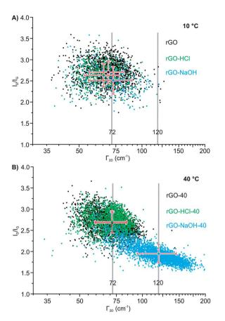
Fig. 2 Raman analysis of the overall quality of (A) rGO, rGO–HCl, and rGO–NaOH and (B) rGO-40, rGO-HCI-40 and rGO-NaOH-40.
