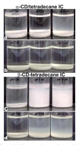
**Fig. 7** Influence of pH of the aqueous solution on the formation of microcrystals of  $\alpha$ -CD–tetradecane ICs (a and b) and  $\beta$ -CD–tetradecane ICs (c and d): images (a) and (c) were captured 24 hours after the initial mixing of CD and tetradecane, while images (b) and (d) were captured after 7 days.
