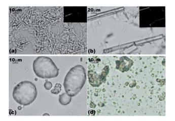
Fig. 12 Optical microscopy images of  $\alpha$ -CD and  $\beta$ -CD hexadecane ICs captured at different times: (a) α-CD-hexadecane IC precipitates immediately after dispersion; (b) α-CD-hexadecane IC microrods after 3 days; (c) β-CD-hexadecane IC structures immediately after dispersion; and (d) β-CD-hexadecane IC microcrystals after 3 days.
