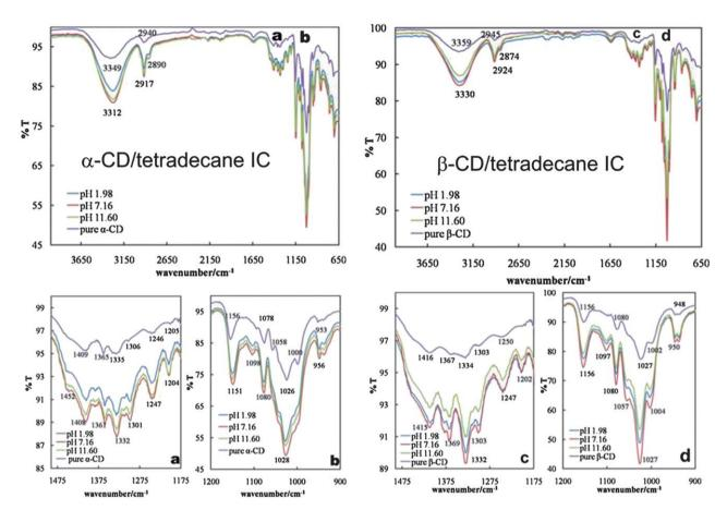
**Fig. 8** LHS images: FT-IR spectra of pure  $\alpha$ -CD and  $\alpha$ -CD-tetradecane ICs prepared in aqueous solutions at different pH. An expanded region labelled (a) and (b) in the main spectra is shown below. RHS images: FT-IR spectra of pure β-CD and β-CD-tetradecane ICs prepared in aqueous solutions at different pH. An expanded region labelled (c) and (d) in the main spectra is shown below.
