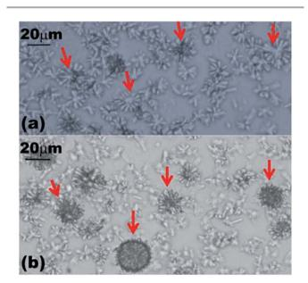
**Fig. 6** Optical images showing the formation of spherical structures by α-CD-tetradecane ICs after dissolving the microrods by heating them at 85 °C before cooling to room temperature. (a) Optical micrographs showing the process of forming spherical structures 5 minutes after the aqueous solution was deposited on the microscope glass slide from a hot bath. (b) The same sample 15 minutes later on the microscope slide.
