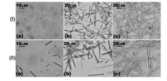
**Fig. 10** Optical micrographs showing the effect of urea concentration on the size of  $\alpha$ -CD-tetradecane IC microrods as a function of time. Row I: in 0.5 M urea (a) immediately after dispersion; (b) after 24 hours; and (c) after 3 days. Row II: in 1 M urea (a) immediately after dispersion; (b) after 24 hours; and (c) after 3 days.
