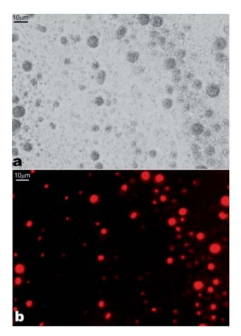
Fig. 13 Images of the β-CD-tetradecane IC structures doped with Nile Red. (a) Optical micrograph; and (b) fluorescence microscopy image with the TRITC filter set. Nile Red fluorescence was observed using the TRITC filter set. Scale bars are 10 μm.
