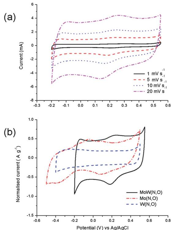
**Fig. 4** Electrochemical characterisation of MoW(N,O) as a supercapacitor electrode material in 1 M  $\text{H}_2\text{SO}_4$  electrolyte. Cyclic voltammograms (third cycle) at various scan rates (a) and CV of the bimetallic oxynitride compared to the cyclic voltammograms of the monometallic compounds at a scan rate of  $5 \text{ mV s}^{-1}$ ; the current is normalised with the weight of the active material (b).
