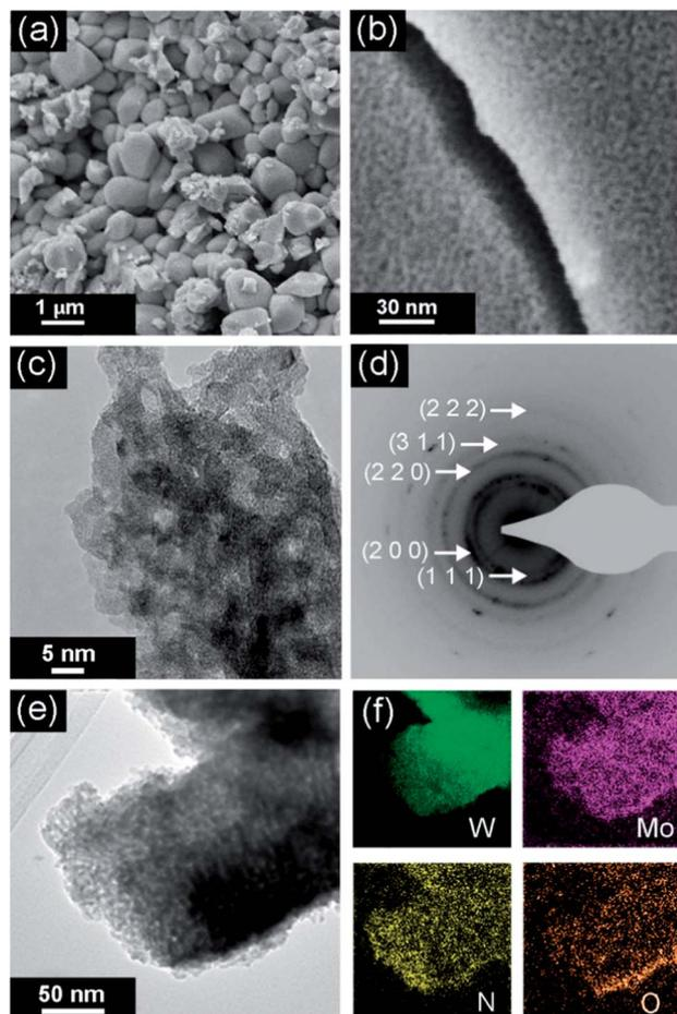
**Fig. 3** Electron microscopy characterisation: SEM images (a and b); bright field TEM image and the electron diffraction pattern (c and d); a TEM image and the corresponding EFTM maps depicting the distribution of W, Mo, N and O elements (e and f).
