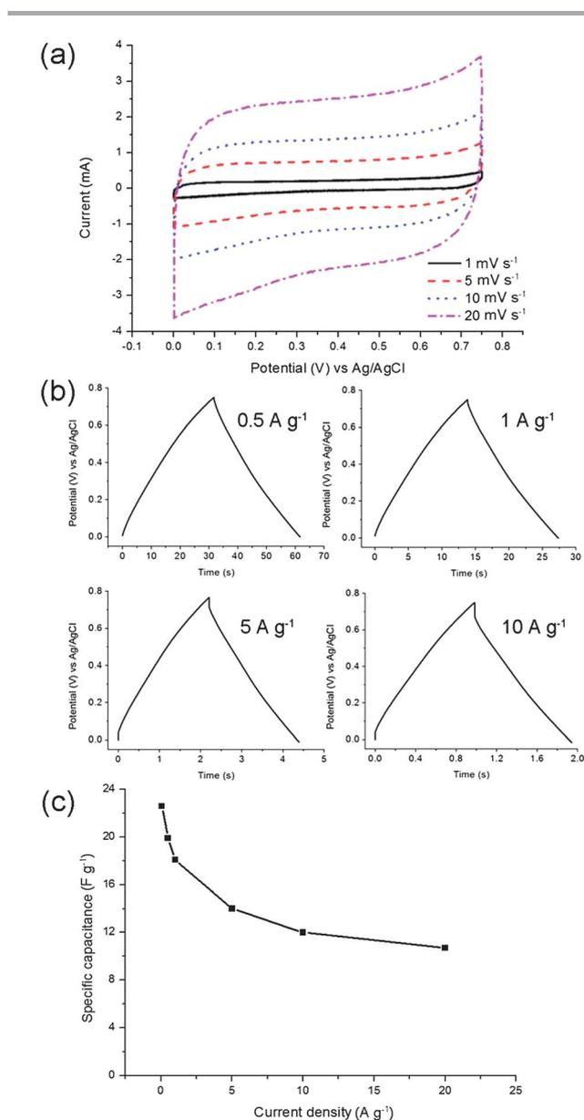
**Fig. 8** Molybdenum tungsten oxynitride electrodes in a symmetric cell. Cyclic voltammetry measurements at the scan rates of 1, 5, 10 and 20  $\text{mV s}^{-1}$  (a); galvanostatic charge and discharge curves at different current densities (b); the rate capability at the current densities between 0.05 and 20  $\text{A g}^{-1}$  (c).
