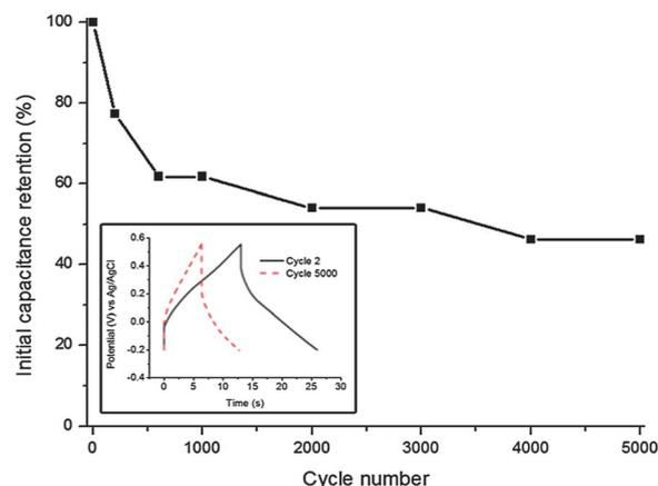
**Fig. 6** Cyclic stability of molybdenum tungsten oxynitride in 1 M H<sub>2</sub>SO<sub>4</sub> electrolyte cycled at a current load of 5 A g<sup>-1</sup>: initial capacitance retention and galvanostatic charge and discharge curves (inset).
