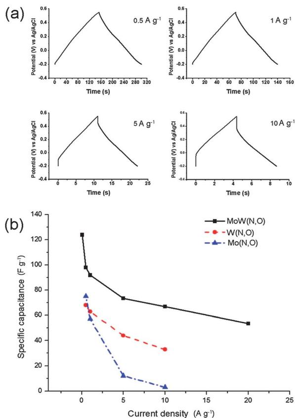
**Fig. 5** Galvanostatic charge and discharge curves of molybdenum tungsten oxynitride (a) and its rate capability in 1 M H<sub>2</sub>SO<sub>4</sub> electrolyte (b). Rate capabilities of molybdenum and tungsten oxynitrides are given for comparison in (b).
