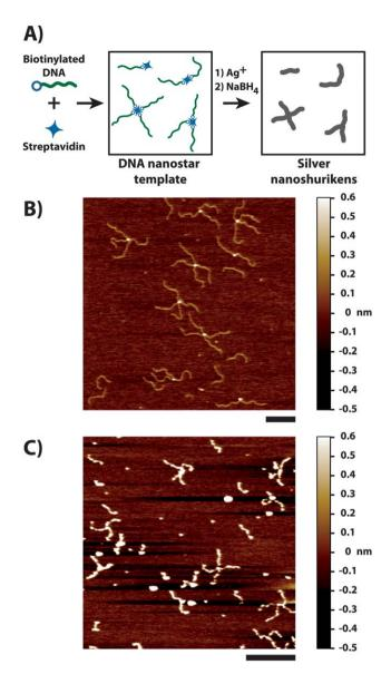
**Fig. 1** (A) A monobiotinylated 541bp DNA (B-DNA541, 49 nM) is assembled with streptavidin (16.3 nM) in NaCl solution (0.2 M) prior to 100-fold dilution in water and addition of AgNO $_3$  (50  $\mu$ M) and NaBH $_4$  (50  $\mu$ M). Representative AFM images of the DNA nanostar templates (B) and resulting silver nanostructures after metallization (C). All scale bars are 200 nm.
