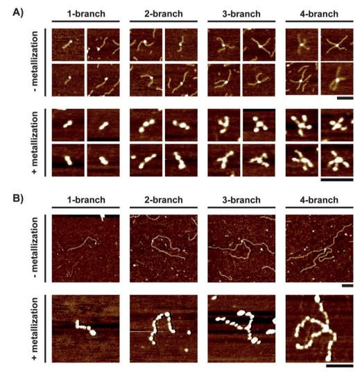
**Fig. 5** AFM images of the four kinds of branched nanostructures before (*top*) and after (*bottom*) silver metallization obtained using a monobiotinylated DNA having (A) 206 bp (B-DNA206, 220 nM) and (B) 978 bp (B-DNA978, 21 nM). Streptavidin concentrations are 40 nM (A) and 3 nM (B). All scale bars are 100 nm. The height scale is the same as that in Fig. 1B and C.
