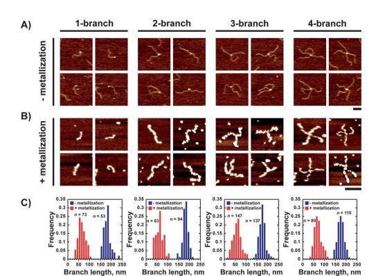
**Fig. 2** AFM images of the four kinds of branched nanostructures before (A) and after (B) silver metallization prepared under the same conditions as in Fig. 1. All scale bars are 100 nm. The height scale is the same as that in Fig. 1B and C. (C) Branch length distributions before (blue) and after (red) metallization for each degree of branching. *n* shows the number of measured branches.
