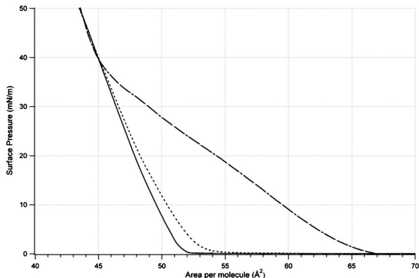
**Fig. 1** (a) Surface pressure-area isotherms of h-DSPC on a aqueous sub-phase [solid line], an aqueous sub-phase containing 20 mM  $\text{CaCl}_2$  sub-phase without [dotted line] and with [dot-dash line] calf-thymus DNA ( $0.067 \text{ mg mL}^{-1}$ ) at  $298 \pm 2 \text{ K}$ . Number of repeats ( $n$ ) = 3.
