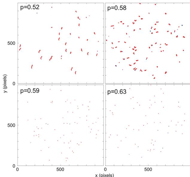
**Fig. 4** Trajectories maps of probe particle movement in hydrogels with  $R = 1$  as the extent of nondegradable polymers is increased from  $p = 0.52$ – $0.63$ . Probe particles are colored coded into two clusters using an F test that determines whether their displacement is statistically significant using a 95% confidence interval.
