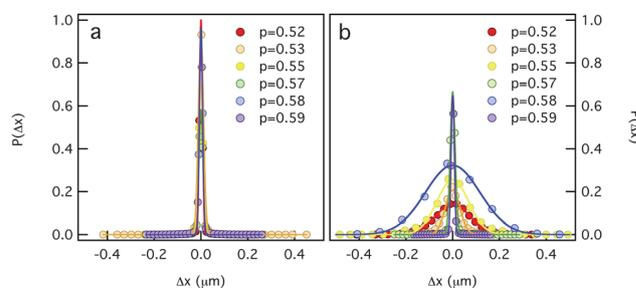
**Fig. 5** Ensemble-averaged van Hove correlation functions for PEG–norbornene hydrogels made with  $R = 1$  and varying the amount of nondegradable cross-links,  $p$ , relative to the peptide cross-linker (a) prior to degradation and (b) after the material has been degraded with  $0.3 \text{ mg mL}^{-1}$  collagenase for 24 h.
