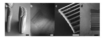
**Fig. 3** (a) SEM image (JEOL 7500F HRSEM) of the microparticles. (b) Interference fringes around such a microparticle in isolation at the air–water interface clearly show the four-lobed quadrupolar deformation of the interface. (c) SEM and (d) microinterferometry of the interface undulations near the ends of a microparticle. The scale bars correspond to 50  $\mu$ m.
