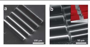
Fig. 6 Shape of the oil-water interface around (a) an isolated microparticle and (b) between two microparticles of differing wavelengths ( $\lambda = 36~\mu m$  and  $60~\mu m$ respectively). The inset in (b) shows the corresponding shape of the interface in surface evolver simulation.
