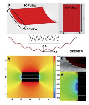
**Fig. 1** (a) Schematic of a particle for Surface Evolver simulation. (b) Iso-height contour of the equilibrium interface around a corrugated particle. (c) Perspective view of the interface shape near the undulated contact line. (d) Iso-height contour of the equilibrium interface in near field close to the corrugated side of the particle. The color code in (d) corresponds to the legend in (b).
