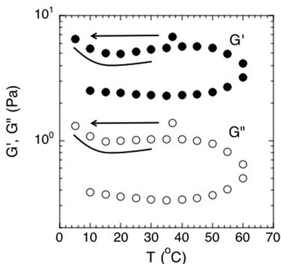
**Fig. 8** Effect of temperature on the elastic and viscous moduli of *S. epidermidis* biofilms at a constant frequency of 1 Hz. Points were extracted from experiments conducted over a frequency range of 0.005–10 Hz. Order of experimentation was 37 °C, then 5 °C to 60 °C increasing at increments of 5, followed by decreasing from 60 °C to 10 °C in increments of 5. Data shown from 1 experiment for purposes of clarity.
