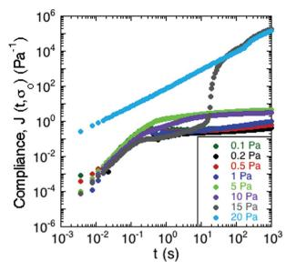
Fig. 5 Creep of S. epidermidis grown in TSB with 86 mM NaCl. A constant stress was applied at t = 0 and the material compliance measured over 20 minutes. Data shown from 1 experiment for purposes of clarity.
