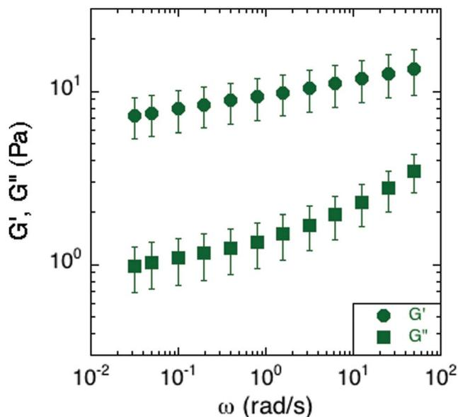
**Fig. 4** Elastic and viscous moduli of *S. epidermidis* biofilms grown in TSB with 86 mM NaCl. This data includes 6 replicates, with each comprised of an average modulus of the experiments conducted at 300 and 250  $\mu\text{m}$  under both compression and tension. Error bars represent the standard error of the mean.
