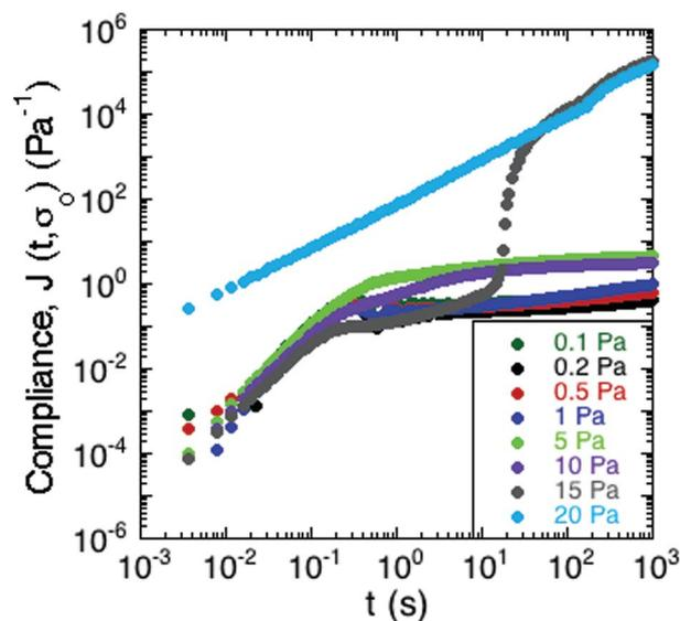
**Fig. 5** Creep of *S. epidermidis* grown in TSB with 86 mM NaCl. A constant stress was applied at  $t = 0$  and the material compliance measured over 20 minutes. Data shown from 1 experiment for purposes of clarity.
