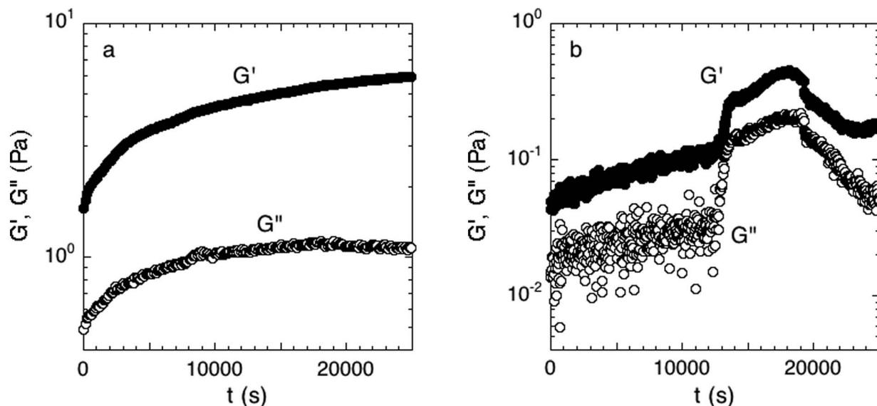
**Fig. 2** (a) Accepted and (b) rejected attachment phase. Measured over 7 hours at 300  $\mu\text{m}$  and a strain of 0.016 directly after the initial growth period. The moduli in the accepted experiment have reached equilibrium while the rejected experiment has not. Examples of one experiment of each case are shown.
