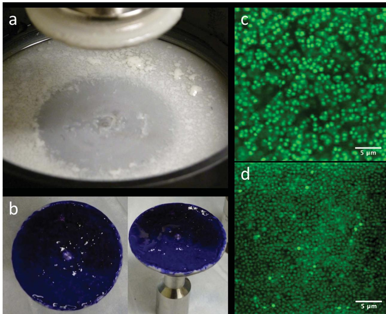
**Fig. 3** (a) Base of rheometer immediately after draining media and lifting the parallel plate. (b) 40 mm diameter parallel plate stained with Gram crystal violet depicting full coverage of biofilm. (c and d) CLSM images of various areas of the biofilm after rheological testing, showing similar morphology throughout.
