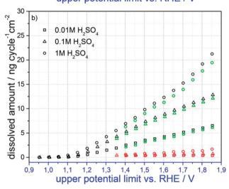
Fig. 4 The amount of dissolved platinum during potential cycling at a scan rate of 0.01 V s<sup>-1</sup> between 0.05 V<sub>RHE</sub> and the corresponding upper potential in (a) HClO<sub>4</sub> and (b) H<sub>2</sub>SO<sub>4</sub> with different concentrations (in black). The red and green color codes show the dissolved amount during the positive and negative sweeps for the corresponding concentrations; ( $\diamondsuit$ ) 5 M, ( $\bigcirc$ ) 1 M, ( $\triangle$ ) 0.1 M and ( $\square$ ) 0.01 M.
