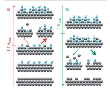
Scheme 1 Alternation of the platinum surface state during: (a) anodic polarization, above ca. 1.1  $V_{\text{RHE}}$  dissolution and passivation of the surface are in competition; and (b) cathodic polarization, during surface reduction below ca. 1.0  $V_{\text{RHE}}$  (re-)deposition and dissolution are in competition.
