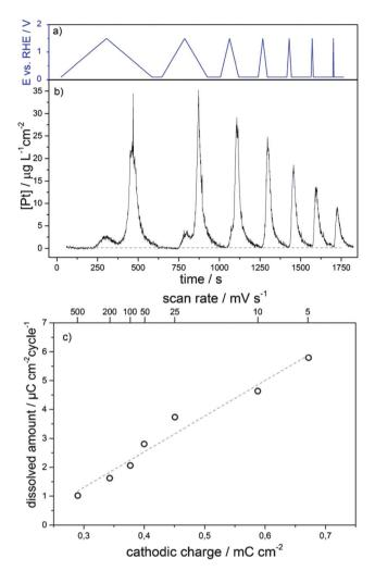
Fig. 2 (a) The applied experimental sequence in 0.1 M HClO<sub>4</sub>; cyclic voltammograms between 0.05 and 1.5 V<sub>RHE</sub> with scan rates of 0.005, 0.01, 0.025, 0.05, 0.1, 0.2, and  $0.5 \text{ V s}^{-1}$ . (b) The corresponding platinum dissolution profile plotted on the same time axis as in (a). The dashed line shows the detection limit for the measurement. (c) The amount of dissolved Pt for each cycle versus the integrated charge for Pt oxide reduction recorded during the same cycle.
