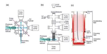
**Fig. 1** Schematic (a) top and (b) side views of the experimental miniature crossed molecular beam machine. (c) The design of the ion optics for DC slice imaging. The red lines represent the electric field lines of force created by the electrodes with applied voltages corresponding to experimental operation. The dimensions of key elements in the scattering region are given in the main text.
