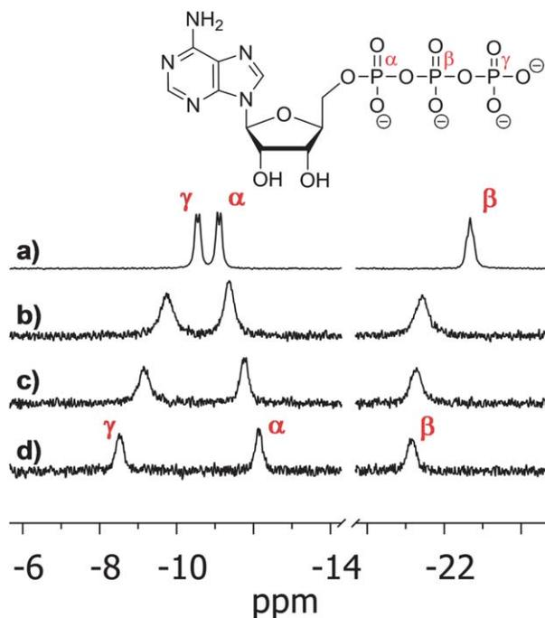
**Fig. 7** <sup>31</sup>P NMR spectra (202 MHz) of ATP (10 mM) in the absence and presence of receptor **1**·Zn<sub>2</sub> in D<sub>2</sub>O at 300 K. (a) [**1**·Zn<sub>2</sub>] = 0. (b) [**1**·Zn<sub>2</sub>] = 0.5 equiv. (c) [**1**·Zn<sub>2</sub>] = 1 equiv. (d) [**1**·Zn<sub>2</sub>] = 2 equiv.
