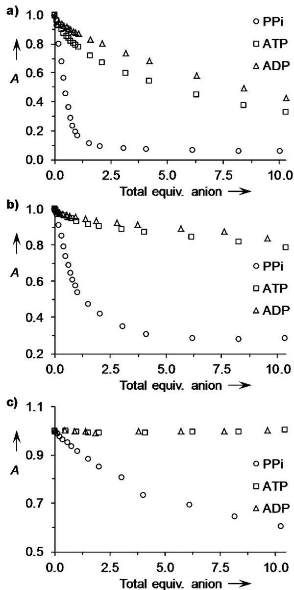
**Fig. 4** Changes in absorbance for 1 : 1 mixtures of (a)  $3\text{-Zn}_2$  : PV (20  $\mu\text{M}$  each) at 640 nm; (b)  $3\text{-Zn}_2$  : PR (20  $\mu\text{M}$  each) at 600 nm and (c)  $3\text{-Zn}_2$  : BPR (10  $\mu\text{M}$  each) at 610 nm; upon addition of up to 10 equiv. of anions (sodium salts) in aqueous solutions of HEPES buffer (5 mM, pH 7.4, 145 mM NaCl) at 25  $^\circ\text{C}$ . A = relative absorbance (arbitrary units).
