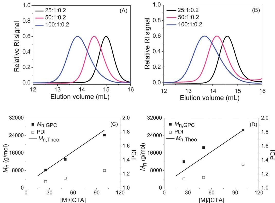
**Fig. 2** GPC RI traces of PCRAMA (A) and PSAMA (B) obtained at different  $[M]/[CDP]$  ratios, and dependence of  $M_n$  and PDI on  $[M]/[CDP]$  ratio for the RAFT polymerization of CRAMA (C) and SAMA (D) in THF at 70 °C.
