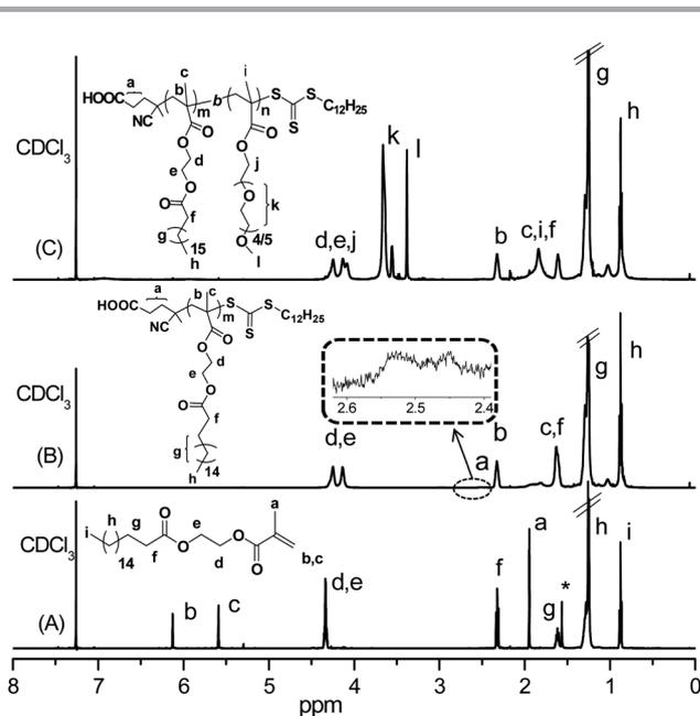
Fig. 1 The <sup>1</sup>H NMR spectra of (A) SAMA, (B) PSAMA and (C) PSAMA-*b*-PMEO<sub>2</sub>MA in CDCl<sub>3</sub>.
