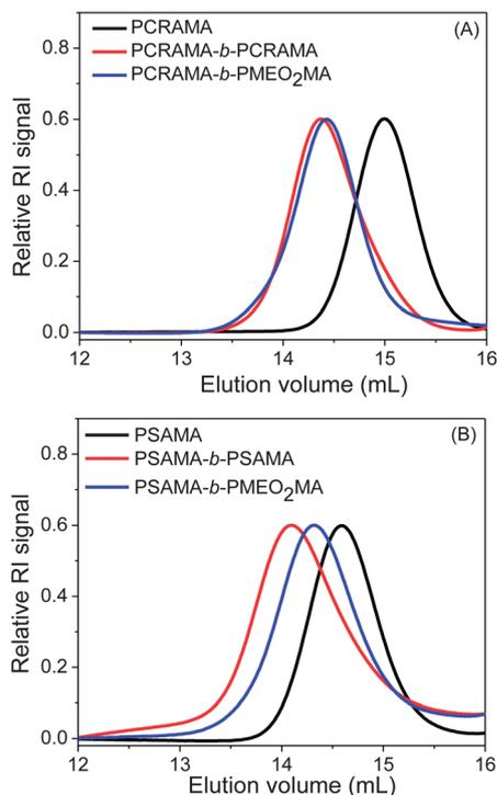
**Fig. 3** GPC RI traces of the (A) PCRAMA-macroCTA, chain extended PCRAMA-*b*-PCRAMA and block copolymer PCRAMA-*b*-PMEO<sub>2</sub>MA; (B) PSAMA-macroCTA, chain extended PSAMA-*b*-PSAMA and block copolymer PSAMA-*b*-PMEO<sub>2</sub>MA.
