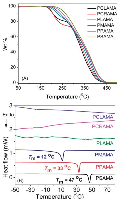
**Fig. 4** TGA thermograms (A) and DSC curves (B) of various side chain fatty acid-containing polymers under N<sub>2</sub> at a heating rate of 10 °C min<sup>-1</sup>.
