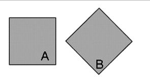
**Fig. 15** Scheme for a chemical diode based on unidirectional propagation of chemical waves. A and B are the excitable media, *i.e.*, the glass plates with ferroin loaded on their surfaces. The waves propagate only from A to B and not *vice versa*.
