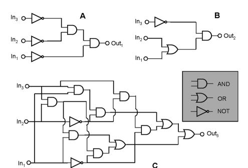
Fig. 5 The three logic circuits that can be implemented through the chromogenic behaviour of SpO. Each circuit has HClO<sub>4</sub>, AlCl<sub>3</sub> and Cu(ClO<sub>4</sub>)<sub>2</sub> as chemical inputs. For the circuits A, B and C the outputs are the absorbance values at 611 nm, 485 nm and 423 nm, respectively.
