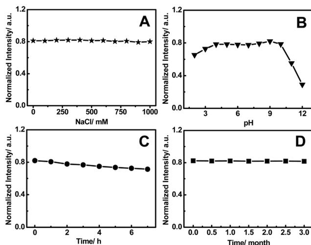
**Fig. 4** (A) The relative fluorescence intensity at  $427\text{ nm}$  (excitation at  $344\text{ nm}$ ) of the FNCPs in the NaCl solution. (B) Dependence of the fluorescence intensity on the pH values from 2 to 12. (C) The variation of the fluorescence intensity of the FNCPs under irradiation by a  $500\text{ W}$  Xe lamp for different time intervals. (D) Photostability of the FNCPs as a function of the storage time.
