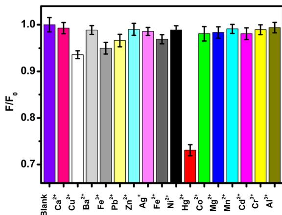
**Fig. 6** Relative fluorescence intensity ( $F/F_0$ ) of the FNCPs in phosphate solutions (25 mM, pH 7.4) with 50  $\mu\text{M}$  different metal ions.  $F$  and  $F_0$  correspond to the fluorescence intensity of the FNCPs with and without 50  $\mu\text{M}$  of different metal ions.
