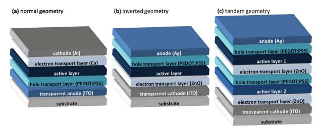
Fig. 6 Schematics of common layer structure of OPV devices in (a) normal, (b) inverted, and (c) tandem geometries with typical materials noted.
