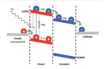
**Fig. 5** Simplified schematic showing the principal internal processes taking place in OPVs. Reproduced from ref. 14, copyright 2010, with permission from Elsevier.
