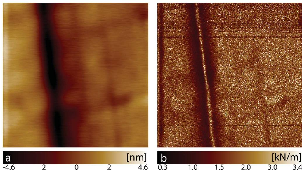
**Fig. 2** Nanoscale modulus mapping of the polished surface of the *M. chuni* sample, produced by the cut perpendicular to the spicule vertical axis: (a) topography map; (b) stiffness map. The map size is  $1 \times 1 \mu\text{m}^2$ .
