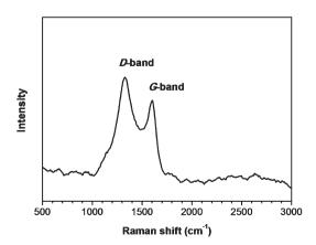
Fig. 3 Raman spectrum of a GCQD sample.
