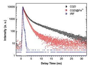
Fig. 8 Fluorescence decay traces of CQDs by TCSPC in the presence (red) and absence (black) of Fe<sup>3+</sup>. The blue line is the instrument response function.
