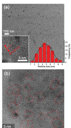
**Fig. 1** (a) TEM image of the as-prepared GCQDs, the insets show a HR-TEM image of a GCQD with graphitic crystalline and the particle size distribution calculated based on 500 nanoparticles. (b) HR-TEM image of the as-prepared GCQDs. The red lines indicate the edges of different nanoparticles.
