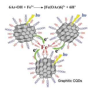
Fig. 7 Schematic illustration of the fluorescence quenching mechanism of the GCQDs in the presence of Fe<sup>3+</sup>. The top equation shows the formation of a complex between Fe3+ and 6 phenolic hydroxyl groups.
