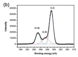
**Fig. 2** (a) Survey X-ray photoelectron spectrum of the GCQDs, only C and O signals are detected. (b) C 1s spectrum of the GCQDs. The C1s spectrum has been deconvoluted into three peaks at 284.6, 286.6 and 288.5 eV, corresponding to C–C, C–O and C=O, respectively.
