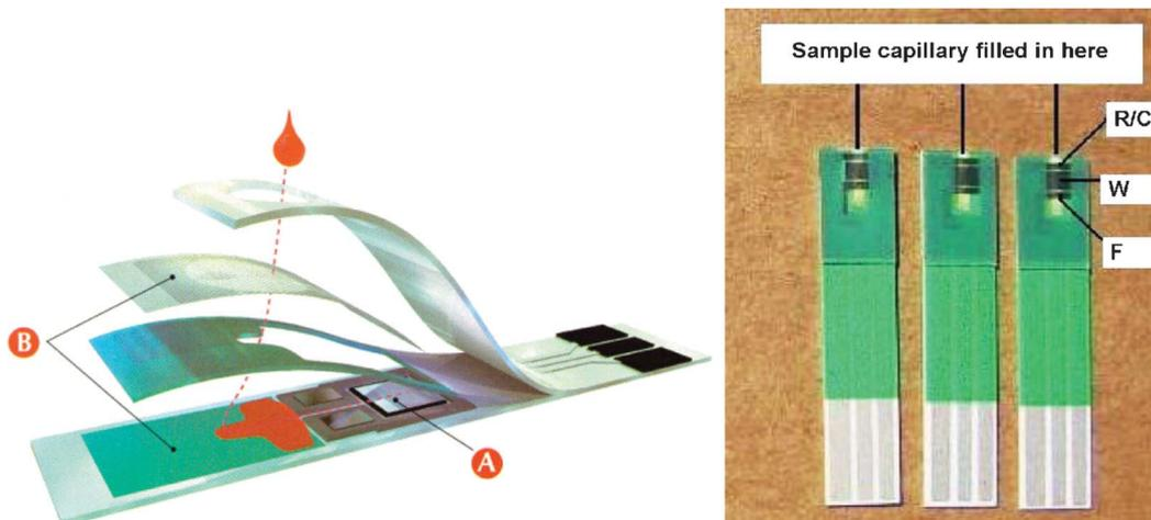
**Fig. 4** Cross section of a commercial strip for self-testing of blood glucose (left, reprinted with permission from ref. 26, copyright 2008, American Chemistry Society) and the test strips designed in 2008 (right, reprinted with permission from ref. 225, copyright 2009, Elsevier).
