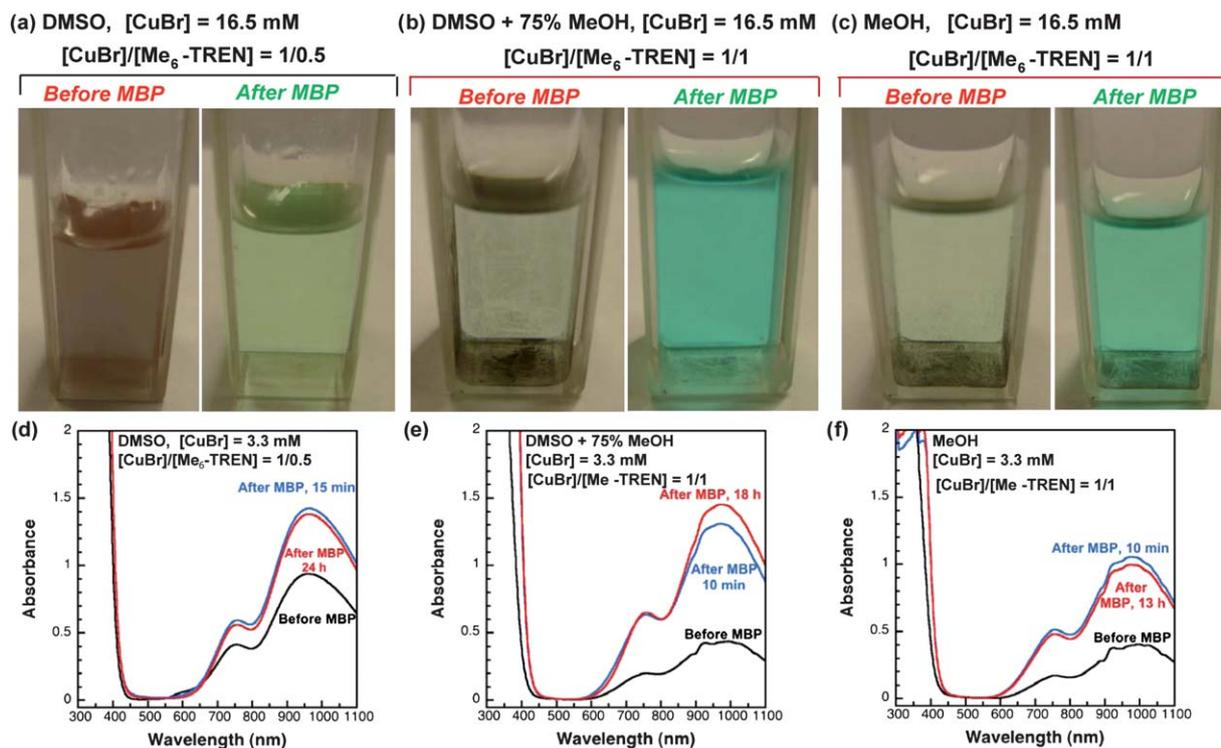
**Fig. 10** Visual observation of Cu(0) nanoparticles and supporting UV-vis spectra of CuBr<sub>2</sub> generated from the disproportionation of CuBr/Me<sub>6</sub>-TREN in DMSO (a and d); DMSO + 75% MeOH (b and e); and MeOH (c and f) before and 10 min after the addition of MBP at 25 °C. Conditions: solvent = 1.8 mL, [MBP]/[CuBr]/[Me<sub>6</sub>-TREN] = 10/1/0.5 (a and d); [MBP]/[CuBr]/[Me<sub>6</sub>-TREN] = 10/1/1 (b, c, e and f); [CuBr] = 16.5 mM (a–c); [CuBr] = 3.3 mM (d–f).
