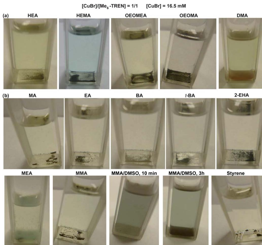
**Fig. 7** Visual observation of Cu(0) nanoparticles generated from the disproportionation of CuBr/Me<sub>6</sub>-TREN in a range of commercial polar monomers (a); and nonpolar monomers (b) at 25 °C. Conditions: monomer = 1.8 mL, [CuBr] = 16.5 mM, [CuBr]/[Me<sub>6</sub>-TREN] = 1/1. Pictures were taken 15 min after mixing reagents, except DMA, which was taken 2 h after mixing the reagents.
