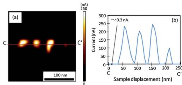
**Fig. 20** (a) A conductive image of the PI film after dot pattern modification. (b) The current profile along C–C' in (a). Reproduced with permission.<sup>32</sup> Copyright 2010, IOP Publishing Ltd.
