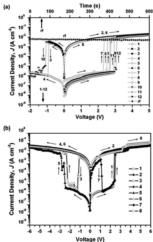
**Fig. 3** (a) The  $J$ – $V$  curve of an ITO/PYTPA-PI/Al sandwich device and (b)  $J$ – $V$  curve of the same device showing bi-directional electrical switching behavior. Reproduced with permission.<sup>10</sup> Copyright 2009, American Institute of Physics.
