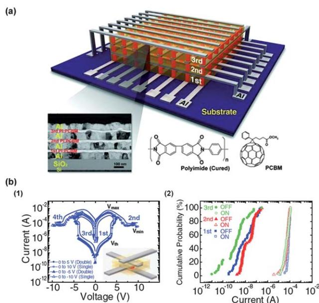
**Fig. 18** (a) A schematic illustration of the three-dimensional PI memory device. The lower part shows the cross-section TEM and the chemical structures of the active materials. (b) (1) Typical  $I$ - $V$  curves of the active layer and (2) cumulative probability data for all operative cells (160 operative cells out of 192 fabricated cells). Reproduced with permission.<sup>19</sup> Copyright 2010, Wiley.
