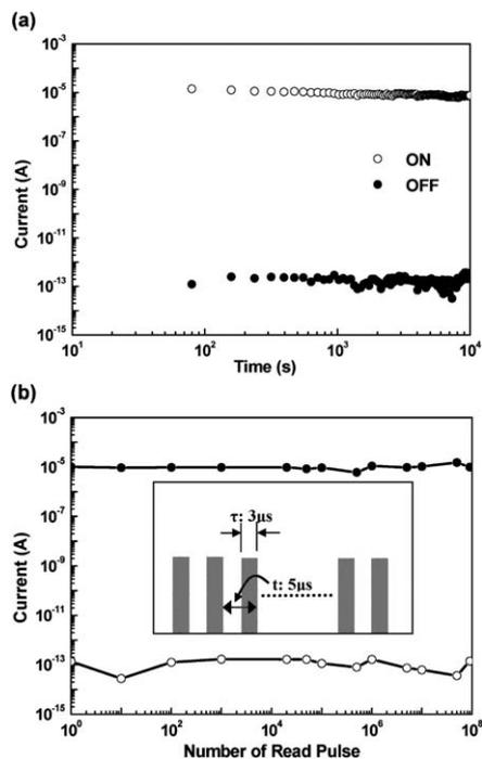
**Fig. 10** (a) Retention times under a continuous readout voltage and (b) the stimulus effect of read pulses on the ON and OFF states of the ITO/PI(APT-6FDA)/Al device. The inset of (b) shows the pulse shapes in the measurement. Reprinted with permission from ref. 16. Copyright 2010, American Chemical Society.
