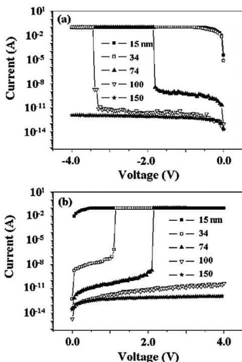
**Fig. 12** *I*-*V* curves of a Au/6F-2TPA PI/Al sandwich device using various thickness (15–150 nm) films; the voltage was swept to both (a) negative and (b) positive directions. Reproduced with permission.<sup>9</sup> Copyright 2009, IOP Publishing Ltd.
