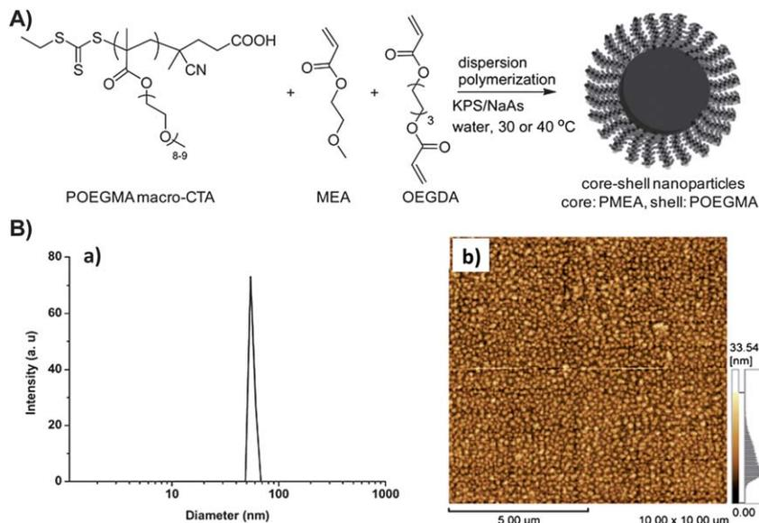
**Fig. 12** (A) Dispersion polymerization of MEA using POEGMA macro-CTA in water. (B) Dynamic light scattering (DLS) result (a) and atomic force microscopy (AFM) graph (b) of the produced cross-linked nanoparticles.<sup>29</sup>
