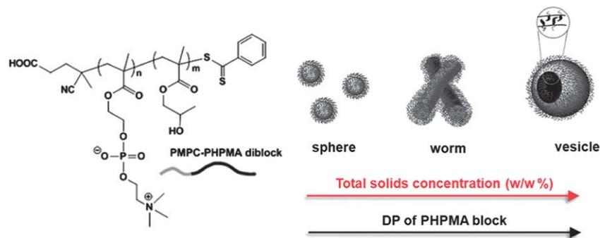
**Fig. 9** Trend relationships of *in situ* formed assemblies with total solids concentration and chain length of the PPHMA block during RAFT aqueous dispersion polymerization of HPMA.<sup>26</sup>
