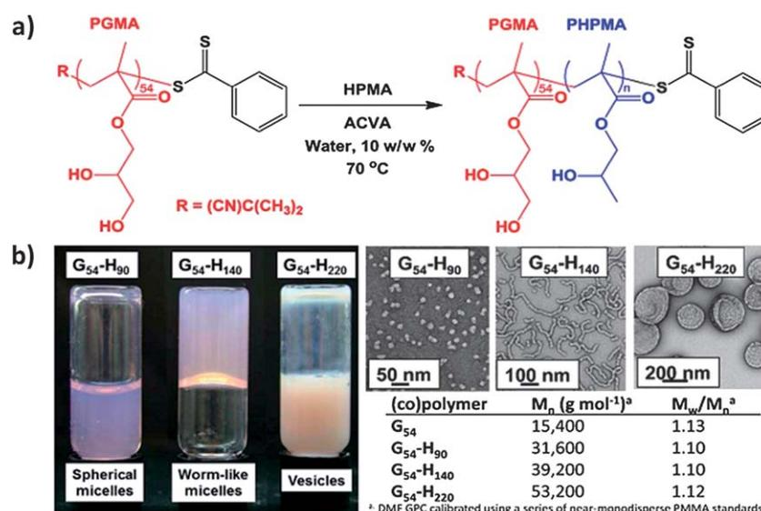
**Fig. 10** (a) RAFT aqueous dispersion polymerization of HPMA monomer using a  $PGMA_{54}$  macro-CTA at 10 wt% and 70 °C. (b) Digital photographs and TEM images of three  $G_{54}\text{-}H_n$  copolymer dispersions with the corresponding molecular weight data.<sup>28</sup>
