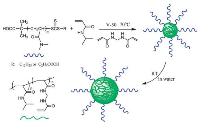
**Fig. 8** RAFT dispersion polymerization of *N*-isopropylacrylamide for the preparation of nanostructured hydrogels.<sup>21</sup>
