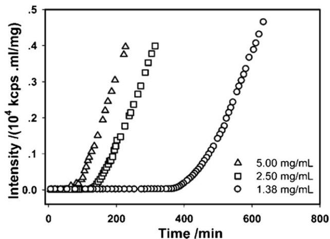
Fig. 4 Time dependence of the scattering intensity of the polymerization-induced self-assembly process at 90° at different PEO macro-CTA concentrations.<sup>12</sup>
