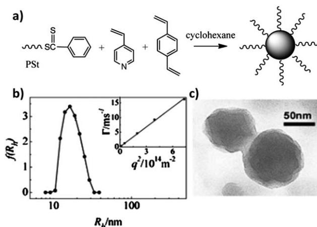
**Fig. 1** (a) Schematic representation for the preparation of core-crosslinked micelles. (b) Hydrodynamic radius distributions of the micelles with cross-linked cores in THF measured by the dynamic light scattering method. The inset shows that  $I/q^2$  is independent of the angle of detection. (c) TEM photo of the core cross-linked micelles.<sup>11</sup>
