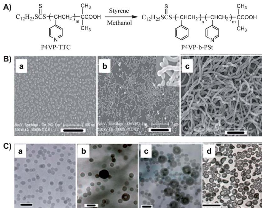
**Fig. 5** (A) RAFT polymerization of styrene in methanol using P4VP-TTC as macro-CTA. (B) FESEM images of the polymeric aggregates prepared by RAFT polymerization for 3 h (a), 4 h (b), and 24 h (c). Scale bar: (a) 500, (b) 2000, (c) 1000 nm. (C) TEM images of the polymeric aggregates with another different feed ratio at different polymerization times: 2 h (a), 4 h (b), 6 h (c), and 24 h (d). Scale bars: (a) 100 nm, (b and c) 200 nm, (d) 1000 nm.<sup>13,15</sup>
