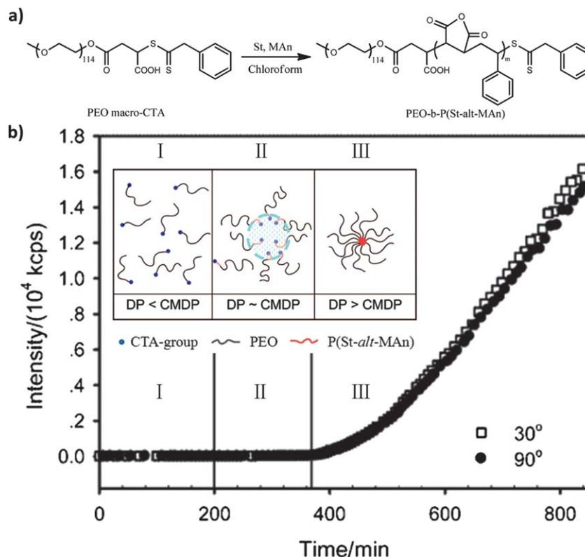
**Fig. 3** (a) RAFT dispersion copolymerization of styrene and maleic anhydride in chloroform with a PEO macro-CTA. (b) Time dependence of the scattering intensity of the polymerization system at scattering angles of 30° and 90°. The inset shows three respective stages during the polymerization-induced self-assembly process.<sup>12</sup>
