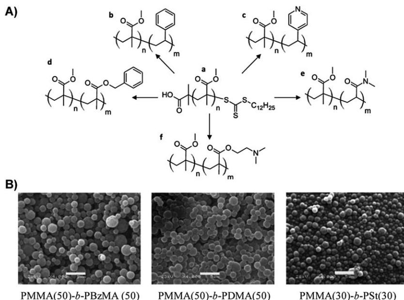
**Fig. 13** (A) The block copolymers synthesized by RAFT dispersion polymerization in  $scCO_2$  from PMMA-RAFT precursors (a): PMMA-*b*-PSt (b), PMMA-*b*-P4VP (c), PMMA-*b*-PBzMA (d), PMMA-*b*-PDMA (e), PMMA-*b*-PDMAEMA (f). (B) SEM of the block copolymer particles. Scale bar in each image is 5  $\mu m$ .<sup>34</sup>
