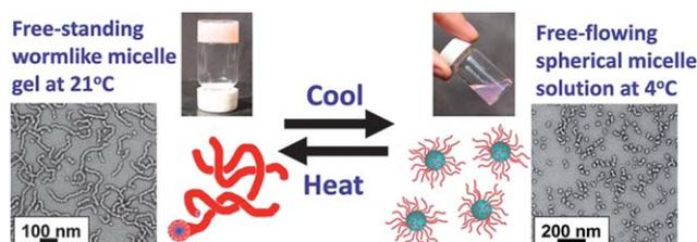
**Fig. 11** Thermoresponsive aqueous solution behavior of a 10 wt% aqueous dispersion of  $G_{54}\text{-}H_{140}$  diblock copolymer particles.<sup>28</sup>
