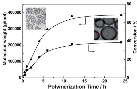
**Fig. 7** The relationship of molecular weights and conversion to the polymerization time. Feed molar ratio: P4VP-TTC/St/AIBN = 10/100 000/1, methanol: 0.9 g, St: 2 g, 80 °C.<sup>16</sup>
