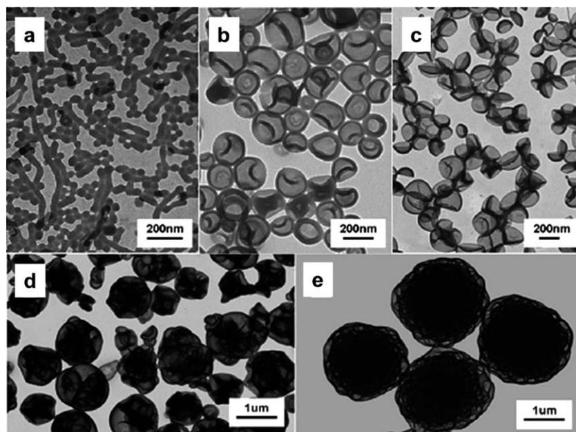
**Fig. 6** TEM images of PAA-*b*-PSt assemblies formed at different molar ratios after 20 h of polymerization. St/PAA-TTC = 250 (a), 500 (b), 750 (c), 1000 (d), and 1250 (e).<sup>19</sup>
