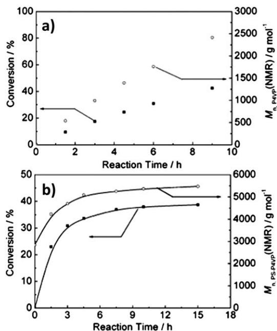
**Fig. 2** Evolution of 4VP conversion and the number-average molecular weights of the P4VP block and the PSt-P4VP with polymerization time in THF (a) and in cyclohexane (b), respectively. There was no cross-linker DVB in either polymerization system.<sup>11</sup>
