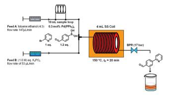
Scheme 2 Suzuki-Miyaura cross coupling under continuous flow conditions.
