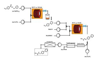
**Fig. 2** Overview of the three-step continuous flow synthesis of biaryl hydrazine intermediate of Atazanavir (3).
