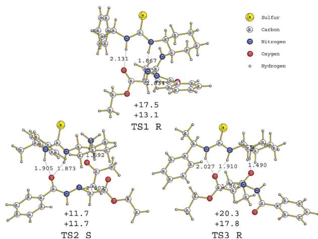
**Fig. 20** Transition state structures located for the enamine (TS1, *R* product) and enol (TS2, *S* product; TS3, *R* product) mechanisms, respectively. Computed at the B3PW91/6-31G(d) (top number) and MP2/6-31G(d)//B3PW91/6-31G(d) (bottom number) levels of theory.
