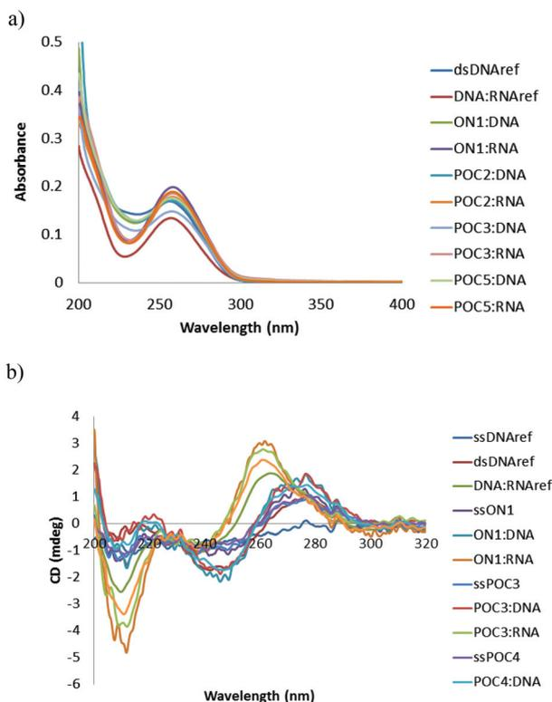
**Fig. 3** Representative UV-Vis (a) and CD spectra (b) of POCs and reference oligonucleotides/duplexes. The spectra were recorded in a medium salt buffer at 19 °C using 2.0  $\mu\text{M}$  concentration of complementary strands.
