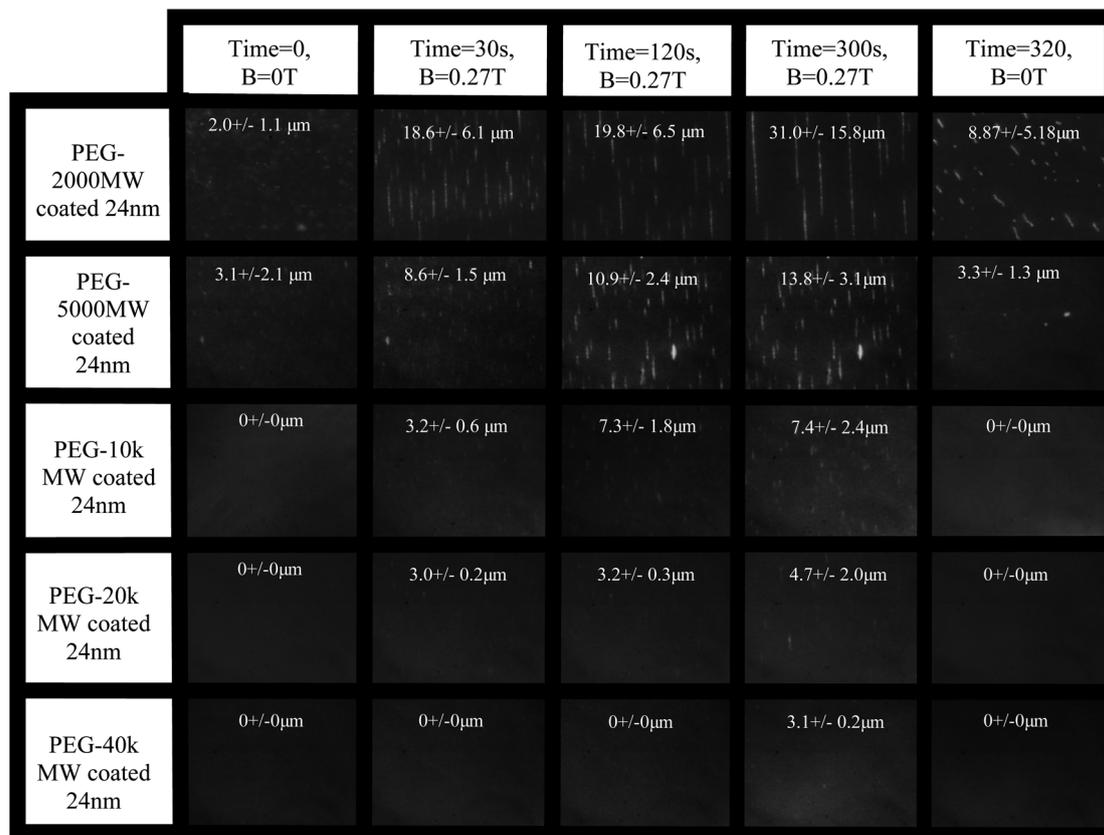
**Fig. 5** Dark field scattering images at varying times for each polymer/particle sample. The average chain length and size distribution has been annotated on each image. It can be seen that the chain length is directly related to the polymer stabilizing brush. The field of view in each image is about 160 microns.
