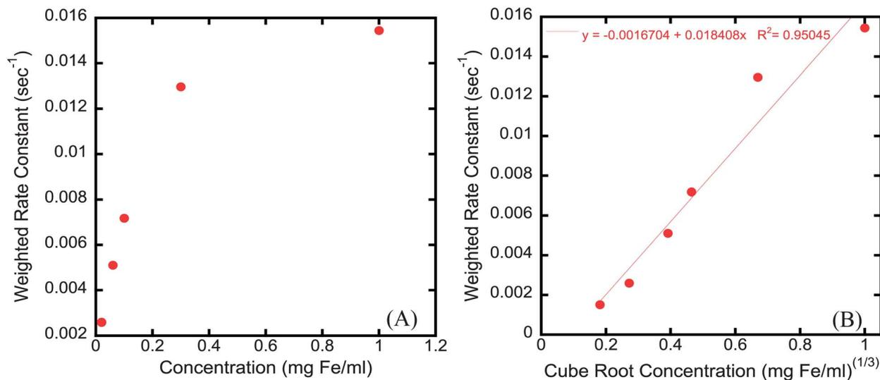
**Fig. 9** (A) Graph of weighted rate constant ( $A_w$ ) versus nanoparticle concentration and (B) weighted rate constant ( $A_w$ ) versus cubic root of concentration correlating the rate at which particles form linear aggregates to interparticle spacing.
