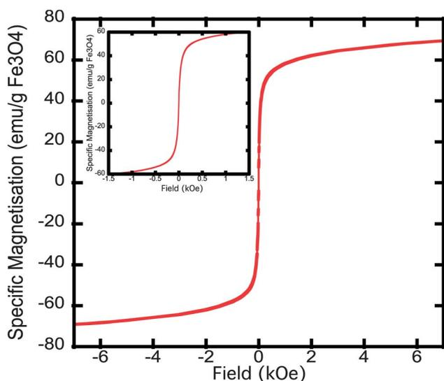
**Fig. 4** Hysteresis loop of the magnetic nanoparticles at 300 K. Specific magnetization is measured in units of emu g<sup>-1</sup> of magnetite as determined by iron analysis of samples using ICP-OES.
