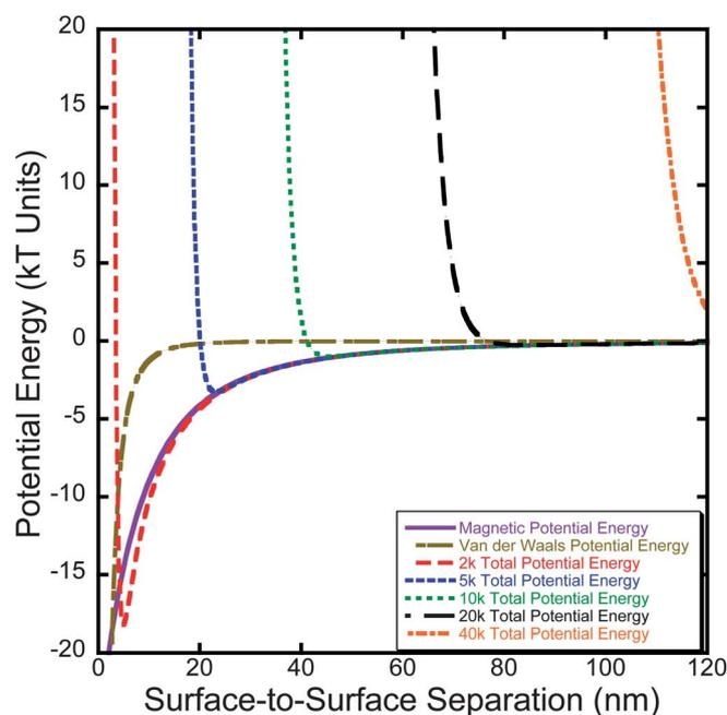
**Fig. 10** DLVO modeling of particle series based upon the total potential energy of each system.  $R_H$  is the hydrodynamic radius,  $R_c$  is the nanoparticle core radius from TEM,  $\Delta_{CC}$  is the core-to-core separation distance, and  $\Delta_{SS}$  is the surface-to-surface separation. For these samples, the polymer layer does not provide sufficient steric repulsion to overcome magnetic and van der Waals attractive forces until 20 000 Da molecular weight.
