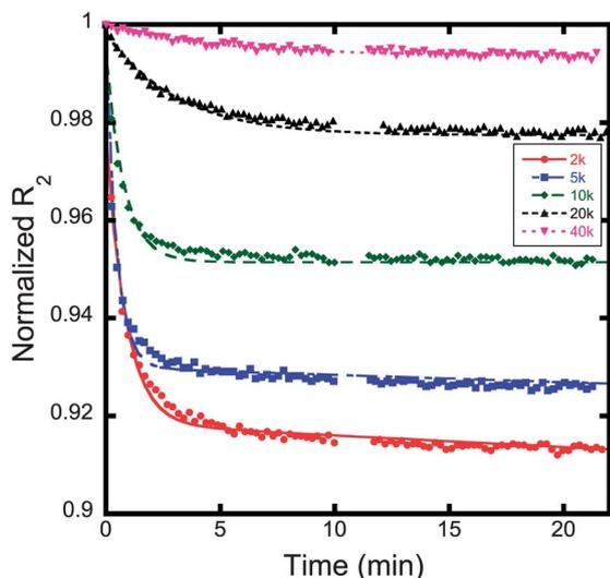
**Fig. 7** Graph of normalized  $R_2$  versus time for varying polymer coated magnetite nanoparticles. The amount of time dependence for each sample decreases as a function of increasing molecular weight. The decay rate for each sample was fit using a biexponential decay function, as displayed in eqn (1). The weighted decay rates are presented in Fig. 8.
