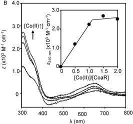
Fig. 1 (A) Titration of coa-O/P DNA (10 nM) with recombinant CoaR monitoring fluorescence anisotropy. (B) Apo-subtracted difference spectra upon anaerobic titration of recombinant CoaR (4.7 µM) with Co(II). Inset shows the Co(II)-dependent change in absorbance at 310 nm.
