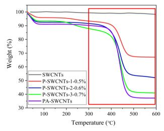
Fig. 6 TGA curves of commercial SWCNTs, P-SWCNTs and PA-**SWCNTs**
