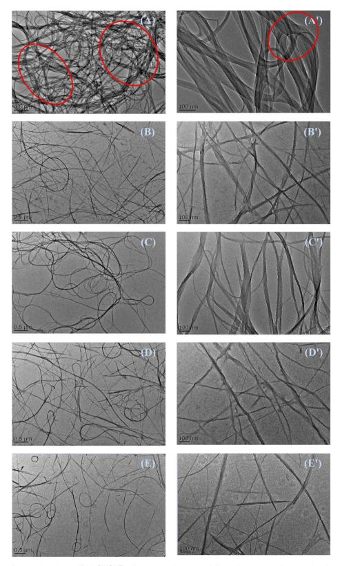
Fig. 7 TEM images of water-based modified SWCNTs dispersions drop-casted from the water solutions, showing different dispersion morphologies. (A): Commercial SWCNTs, (B): P-SWCNTs-0.5%, (C): P-SWCNTs-0.6%, (D): P-SWCNTs-0.7%, (E): PA-SWCNTs. (A') to (E') is the magnification of (A) to (E).
