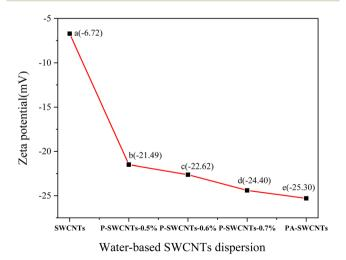
Fig. 4 Relation between zeta potential and water-based SWCNTs dispersion modified by different dispersant. a: Commercial SWCNTs, b: P-SWCNTs-0.5%, c: P-SWCNTs-0.6%, d: P-SWCNTs-0.7%, e:PA-SWCNTs.
