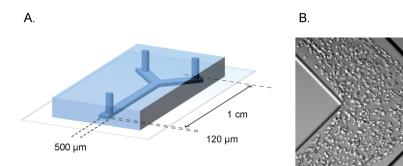
Fig. 1 Microfluidic device for defined engineering of vascular structures. A. Schematic overview of the polydimethylsiloxane-glass device showing the dimensions and geometry of the microchannel. B. Bright field micrograph of the cell suspension inside the microchannel, one hour after seeding
