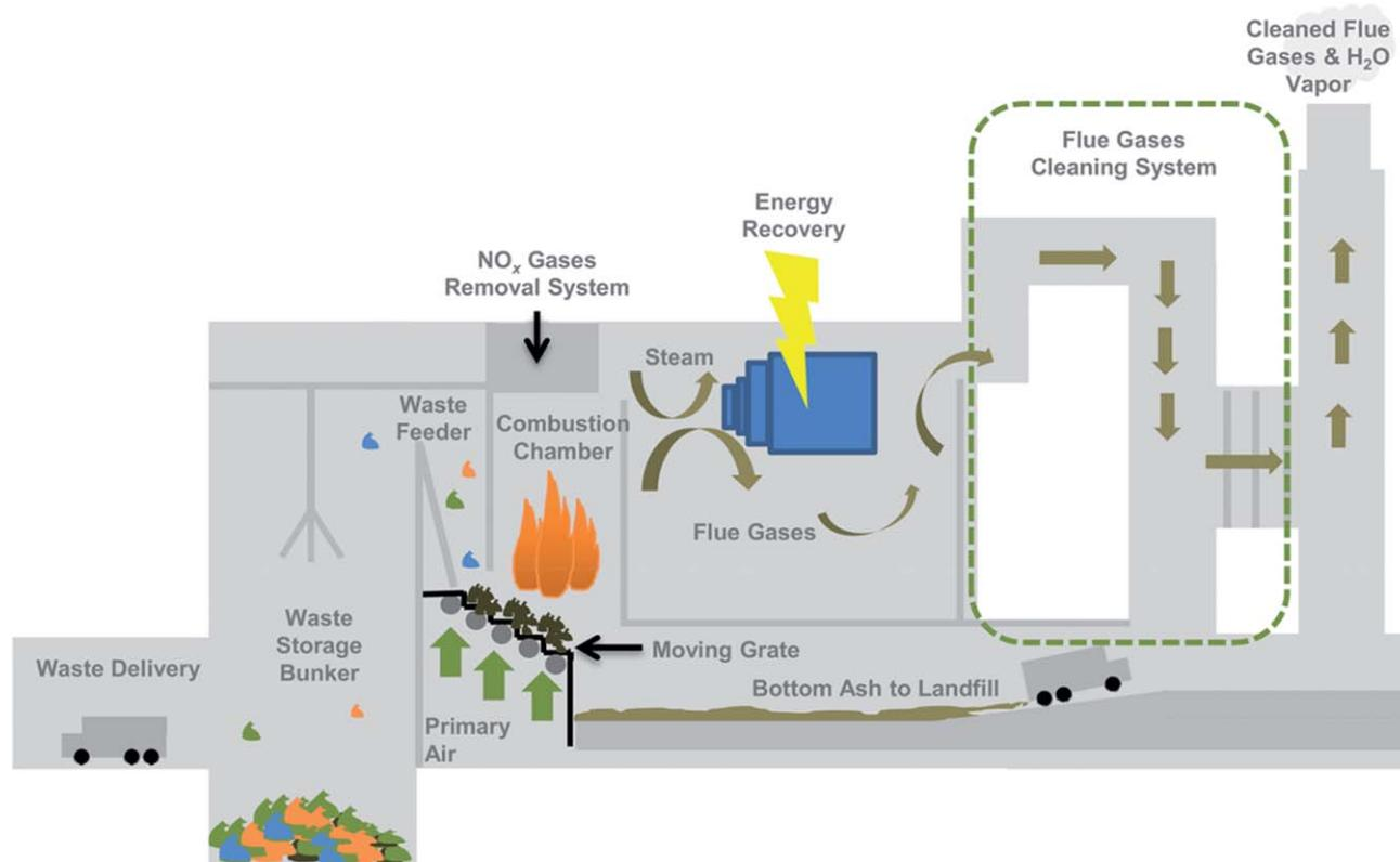
Fig. 1 Schematic of grate incinerator operation.<sup>56</sup>
