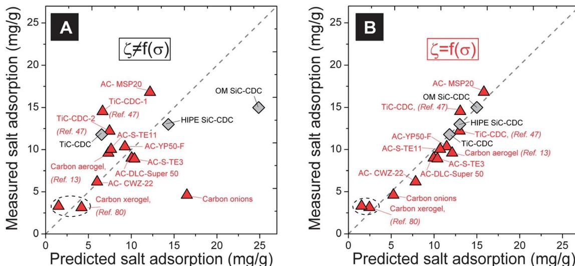
**Fig. 6** Parity plots for salt adsorption ( $c_{\infty} = 5$  mM,  $V_{\text{cell}} = 1.2$  V) for three carbide-derived carbons (grey diamonds) and twelve other materials (red triangles) per gram of carbon in both electrodes combined. (A) Salt adsorption capacity  $\zeta$  assumed independent of pore size  $\sigma$ . (B) Optimized  $\zeta(\sigma)$ -function, see Fig. 4.
