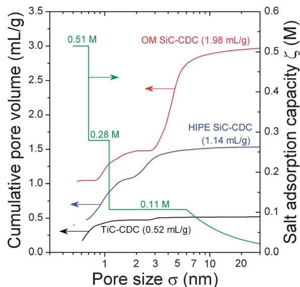
**Fig. 4** Cumulative pore size distributions calculated from QSDFT models of the three tested CDC-materials, as well as the suggested correlation function for the ion adsorption capacity,  $\zeta(\sigma)$ . PSD curves shifted up by  $0.4 \text{ mL g}^{-1}$  for HIPE SiC-CDC and  $1.0 \text{ mL g}^{-1}$  for OM SiC-CDC.
