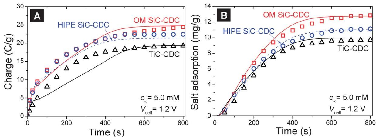
**Fig. 7** (A) Kinetics of charge transfer during the adsorption step and (B) salt electroadsorption in CDI, as a function of time for OM SiC-CDC (squares), HIPE SiC-CDC (circles) and TiC-CDC (triangles). Lines are fits using two-dimensional porous electrode theory.
