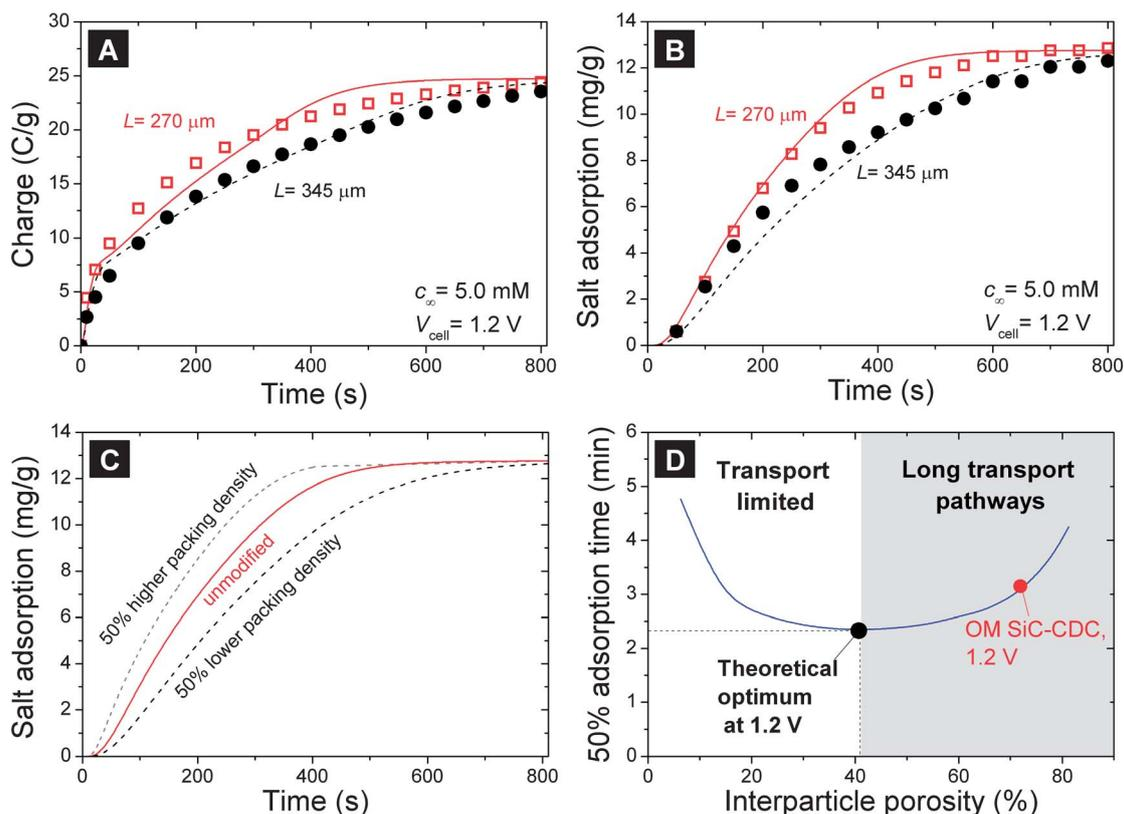
**Fig. 8** (A) Salt electroadsorption and (B) charge transfer during the electroadsorption step in CDI, as a function of time and electrode thickness,  $L$ , for electrodes made of OM SiC-CDC. Lines are predictions using two-dimensional porous electrode theory. (C and D) Calculation results as a function of electrode packing density.
