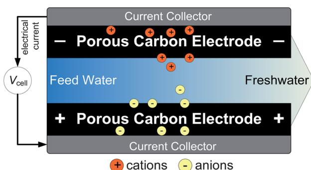
**Fig. 1** Schematic illustration of desalination *via* capacitive deionization (CDI). Upon applying a cell voltage between the two electrodes, anions and cations are electrosorbed within highly porous carbon electrodes to counterbalance the electrical charge. This immobilization of ions decreases the salt concentration in the flow channel, and results in the production of freshwater.
