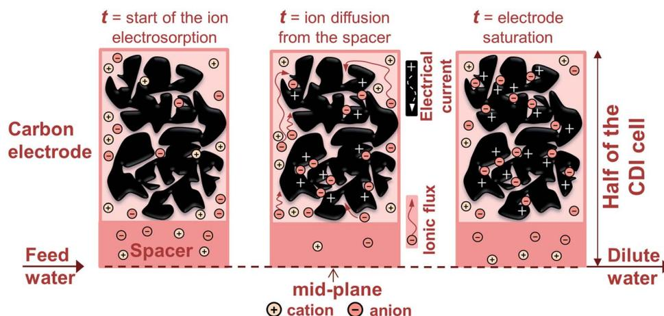
**Fig. 2** Schematic view of the time-dependent two-dimensional porous electrode model, combining a sequence of sub-cells in the flow direction, with ion fluxes into the electrode. A symmetric CDI geometry is assumed, thus only half of a cell is depicted. The electrode contains an electrolyte-filled volume allowing for ion transport, and carbon material in which ions and charge are stored. Electrical current (denoted by “+”) flows through the conductive carbon material.
