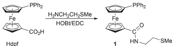
**Scheme 2** Preparation of amidophosphine **1** (HOBT = 1-hydroxybenzotriazole, EDC = 1-ethyl-3-[3-(dimethylamino)propyl]carbodiimide).
