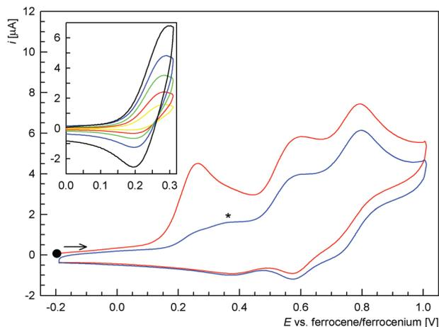
**Fig. 4** Cyclic voltammogram of **1** recorded in 1,2-dichloroethane on a glassy carbon electrode (first scan in red, second scan in blue). The signal marked with an asterisk is presumably due to **10**. The inset shows partial cyclic voltammograms recorded at different scan rates (yellow  $0.02 \text{ V s}^{-1}$ , red  $0.05 \text{ V s}^{-1}$ , green  $0.10 \text{ V s}^{-1}$ , blue  $0.20 \text{ V s}^{-1}$ , and black  $0.50 \text{ V s}^{-1}$ ).
