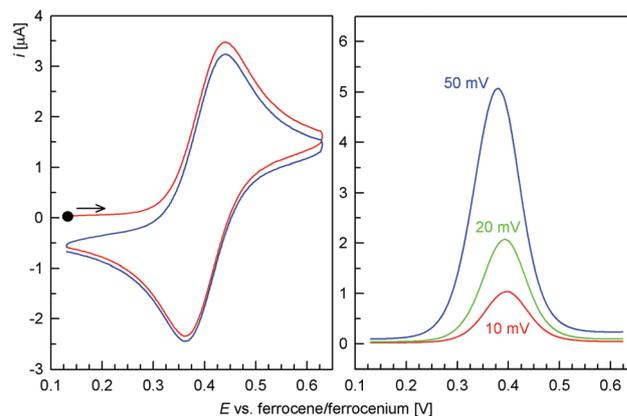
**Fig. 6** Representative cyclic (left; scan rate  $0.1 \text{ V s}^{-1}$ ) and differential pulse (right) voltammograms of **10** recorded in 1,2-dichloroethane on a glassy carbon electrode. The voltammograms are presented with the same scale; modulation amplitude for the differential pulse voltammograms is given in the figure.
