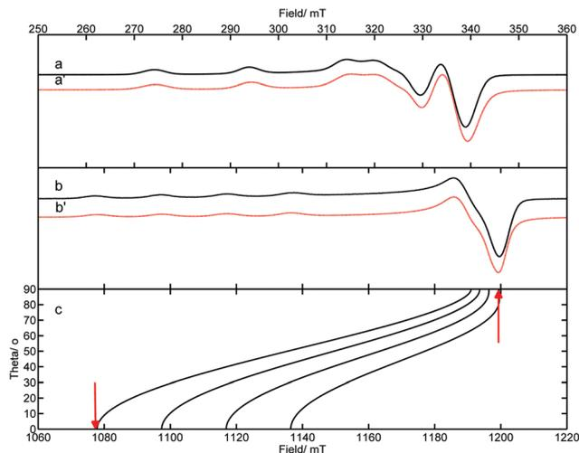
**Fig. 3** CW EPR spectra (10 K) of  $[\text{Cu}(\text{en})_2](\text{OTf})_2$  **1** recorded in a frozen acetonitrile-THF (1 : 1) solution (a) X-band, (b) Q-band, (c) road-map showing the angular dependency profile. The corresponding simulations are given in a' and b'.
