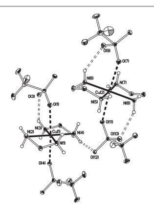
**Fig. 1** Displacement ellipsoid plot (35%) of [Cu(en)<sub>2</sub>](OTf)<sub>2</sub>. H atoms omitted for clarity, except those bonded to N, which are shown as spheres of arbitrary radius.
