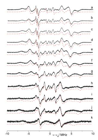
**Fig. 5** CW Q-band <sup>1</sup>H ENDOR spectra (10 K) of [Cu(en)<sub>2</sub>](OTf)<sub>2</sub> **1** recorded at the field positions (a) 1198, (b) 1193.5, (c) 1188.9, (d) 1183.6, (e) 1175.9, (f) 1164.7, (g) 1151.6, (h) 1135.2, (i) 1116.2, (j) 1095.6 and (k) 1077.5 mT. Corresponding simulations are shown with a dotted line.
