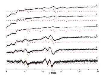
**Fig. 4** CW Q-band <sup>14</sup>N ENDOR spectra (10 K) of [Cu(en)<sub>2</sub>](OTf)<sub>2</sub> **1** recorded in a frozen  $d^3$ -acetonitrile– $d^8$ -THF (1:1) solution. The ENDOR spectra were recorded at the field (a) 1198, (b) 1193.5, (c) 1188.9, (d) 1135.2, (e) 1095.6 and (f) 1077.5 mT. Corresponding simulations are shown with a dotted line. Peaks appearing at lower frequencies arise from solvent  $^2$ H.
