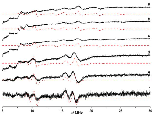
**Fig. 4** CW Q-band  $^{14}\text{N}$  ENDOR spectra (10 K) of  $[\text{Cu}(\text{en})_2](\text{OTf})_2$  **1** recorded in a frozen  $d^3$ -acetonitrile- $d^8$ -THF (1 : 1) solution. The ENDOR spectra were recorded at the field (a) 1198, (b) 1193.5, (c) 1188.9, (d) 1135.2, (e) 1095.6 and (f) 1077.5 mT. Corresponding simulations are shown with a dotted line. Peaks appearing at lower frequencies arise from solvent  $^2\text{H}$ .
