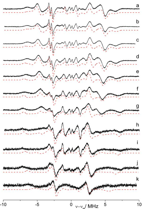
**Fig. 5** CW Q-band  $^1\text{H}$  ENDOR spectra (10 K) of  $[\text{Cu}(\text{en})_2](\text{OTf})_2$  **1** recorded at the field positions (a) 1198, (b) 1193.5, (c) 1188.9, (d) 1183.6, (e) 1175.9, (f) 1164.7, (g) 1151.6, (h) 1135.2, (i) 1116.2, (j) 1095.6 and (k) 1077.5 mT. Corresponding simulations are shown with a dotted line.
