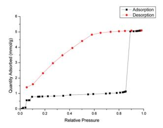
Fig. 4 Water vapour sorption isotherm on Fe<sub>6</sub>Ca<sub>2</sub>(SeO<sub>3</sub>)<sub>9</sub>Cl<sub>4</sub> at 293 K, see text for explanation.
