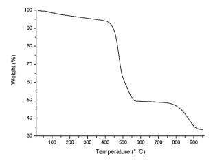
Fig. 3 TG curve of Fe<sub>6</sub>Ca<sub>2</sub>(SeO<sub>3</sub>)<sub>9</sub>Cl<sub>4</sub> for the range 20 °C to 950 °C, see text for explanation.
