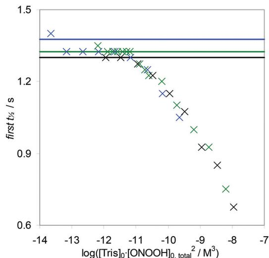
**Fig. 7** Decomposition of 0.047 mM (blue), 0.25 mM (green) and 0.34 mM (black) peroxynitrite at pH = 6.8 in 0.1 M phosphate buffers with varied Tris concentrations. The solid horizontal lines indicate the first half-life of the absorbance of peroxynitrite in the absence of Tris. When  $[\text{Tris}]_0[\text{ONOO}^-]_{0,\text{total}}^2$  exceeds  $6.3 \times 10^{-12} \text{ M}^3$ , Tris significantly catalyses the disproportionation.
