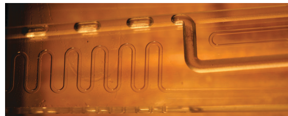
Fig. 5 Formation of the Taylor flow regime in a glass micro-mixer prior to the washcoated microchannel reactor.
