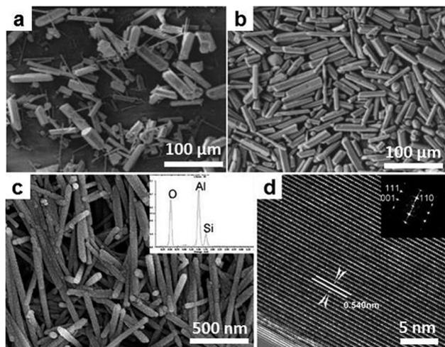
**Fig. 9** Whiskers of complex oxides by SMS. (a and b) SEM images of HPA whiskers produced by seeded growth in  $K_2SO_4$  at  $1300\text{ }^\circ\text{C}$ . (Reprinted with permission from ref. 111. Copyright 2001 John Wiley and Sons.) (c) SEM and (d) HRTEM images of mullite whiskers synthesized in a  $B_2O_3$  doped molten salts system. (Reproduced from ref. 116 with permission from The Royal Society of Chemistry.)
