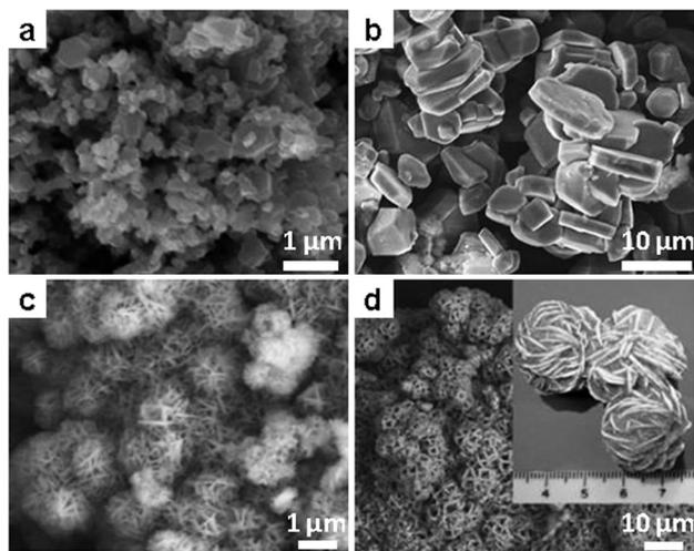
**Fig. 8** LiCoO<sub>2</sub> nanostructures by SMS. (a and b) SEM images of LiCoO<sub>2</sub> particles synthesized from LiCl and Co(NO<sub>3</sub>)<sub>2</sub> in LiNO<sub>3</sub> at 650 °C and 850 °C. (Reprinted with permission from ref. 81. Copyright 2005 Elsevier.) (c and d) SEM images of the “desert rose” shaped LiCoO<sub>2</sub> nanostructures synthesized in hydroxide melt at 200 °C for 24 h and 48 h. (Reprinted with permission from ref. 83. Copyright 2008 John Wiley and Sons.)
