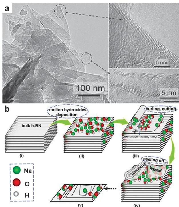
**Fig. 17** Exfoliation of bulk h-BN with molten hydroxides. (a) TEM images for the h-BN nanosheets exfoliated in NaOH/KOH melt at 180 °C. (b) Schematic illustration of the exfoliation mechanism based on a self-curling and peeling off process. (Reprinted with permission from ref. 155. Copyright 2013 John Wiley and Sons.)
