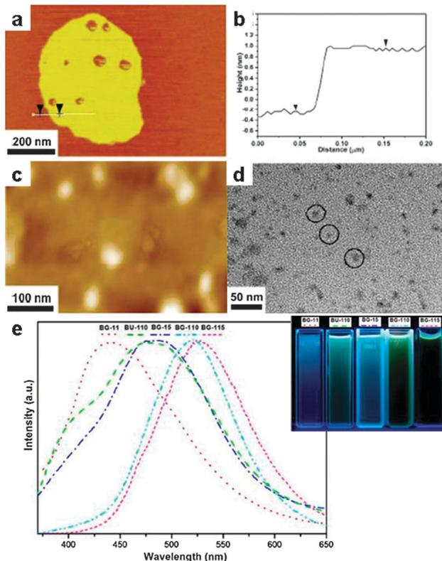
**Fig. 18** BCN nanostructure synthesized in LiCl/KCl with tunable bandgap. (a and b) Atomic force microscopy (AFM) characterization of the BCN nanosheets, (c) AFM and (d) TEM images of BCN NPs synthesized from NaBH<sub>4</sub> and urea. (e) Photoluminescence spectra of the BCN dispersions synthesized under different conditions. (Reprinted with permission from ref. 156. Copyright 2011 American Chemical Society.)
