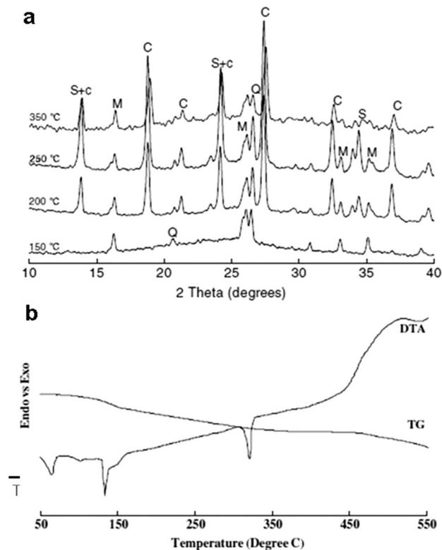
**Fig. 10** Zeolitization of fly ash in NaOH/ $KNO_3$  salt melt. (a) Phase evolution with increasing temperature examined by XRD. C: cancrinite; M: mullite; Q: quartz; S: sodalite. (b) TG-DTA traces of the mixture of fly ash and the salt (NaOH/ $KNO_3$ ). (Reprinted with permission from ref. 119. Copyright 2007 Springer.)
