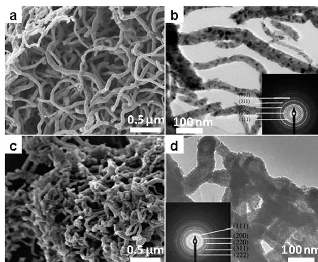
**Fig. 12** Metal carbide nanofibers by templated synthesis using carbon nanotubes in LiCl/KCl. (a and c) SEM and (b and d) TEM images of (a and b) TiC and (c and d) ZrC nanofibers. (Reprinted with permission from ref. 125. Copyright 2009 Elsevier.)
