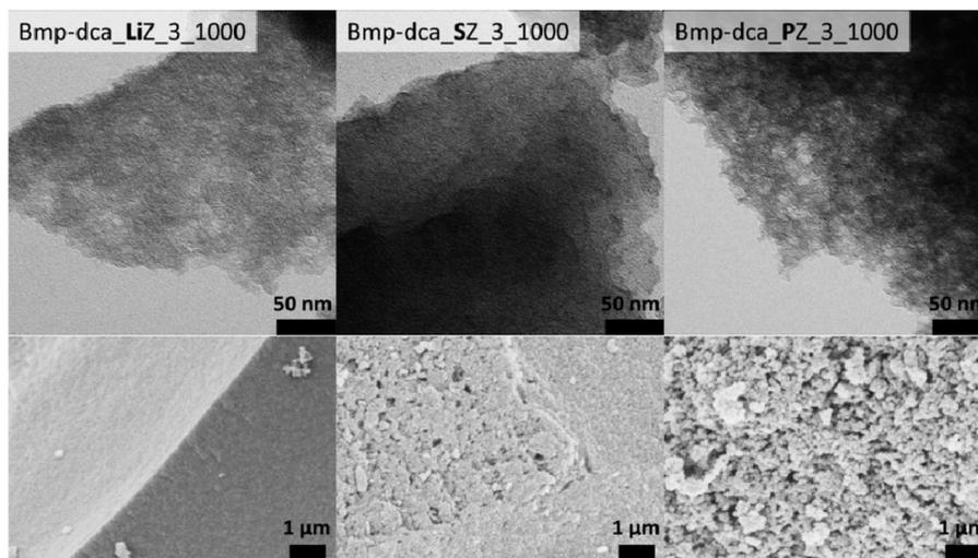
**Fig. 21** TEM (upper row) and SEM pictures (lower row) of nitrogen-doped carbons using Bmp-dca as precursor templated with LiZ (left), SZ (middle) and PZ (right) at equal mass ratios synthesized at 1000 °C. (Reprinted with permission from ref. 170. Copyright 2013 John Wiley and Sons.)
