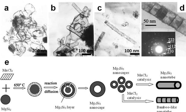
**Fig. 13** TEM images of (a and b)  $\text{Mn}_5\text{Si}_3$  nanocages and (c and d) nanotubes synthesized from  $\text{Mg}_2\text{Si}$  and  $\text{MnCl}_2$ , in which  $\text{MnCl}_2$  was used as both reactants and flux. (e) Schematic illustration of the mechanism for nanocage and nanotube formation. (Reprinted with permission from ref. 132. Copyright 2004 Elsevier.)
