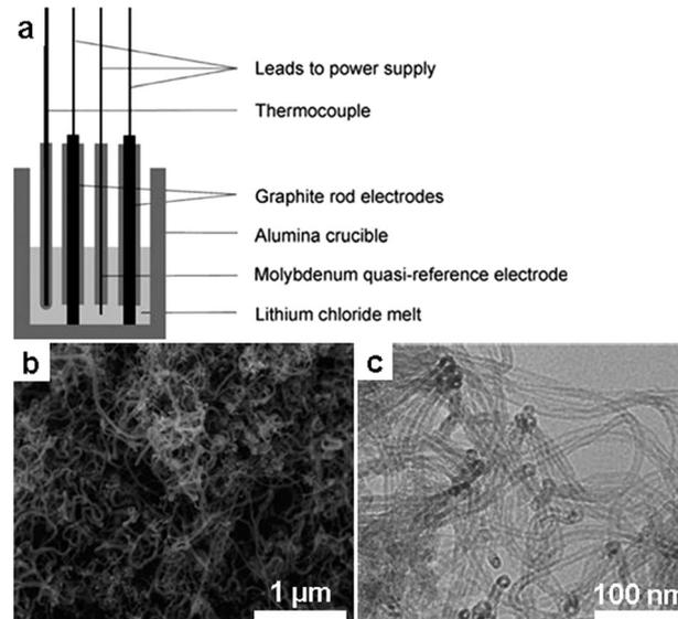
**Fig. 25** CNT production in molten chloride. (a) Schematic of the cell design for the electrolysis of graphite for CNT production. (b) SEM and (c) TEM images of CNTs produced in molten salt. (Reprinted with permission from ref. 196. Copyright 2012 Elsevier.)
