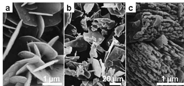
**Fig. 6** SEM images of different phosphates precipitated in  $\text{NaNO}_3$  at  $500\text{ }^\circ\text{C}$  from the salts of the different metal elements: (a)  $\text{Na}_2\text{Zr}(\text{PO}_4)_2$ , (b)  $\text{NaBaPO}_4$  and (c)  $\text{NaCaPO}_4$ . (Reprinted with permission from ref. 67. Copyright 1999 American Chemical Society.)
