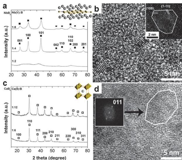
**Fig. 11** Metal borides synthesized in LiCl/KCl from metal chloride and NaBH<sub>4</sub>. (a) XRD pattern and (b) HRTEM image of NbB<sub>2</sub> NCs. (c) XRD pattern and (d) HRTEM image of CaB<sub>6</sub> NCs. (Reprinted with permission from ref. 122. Copyright 2011 John Wiley and Sons.)
