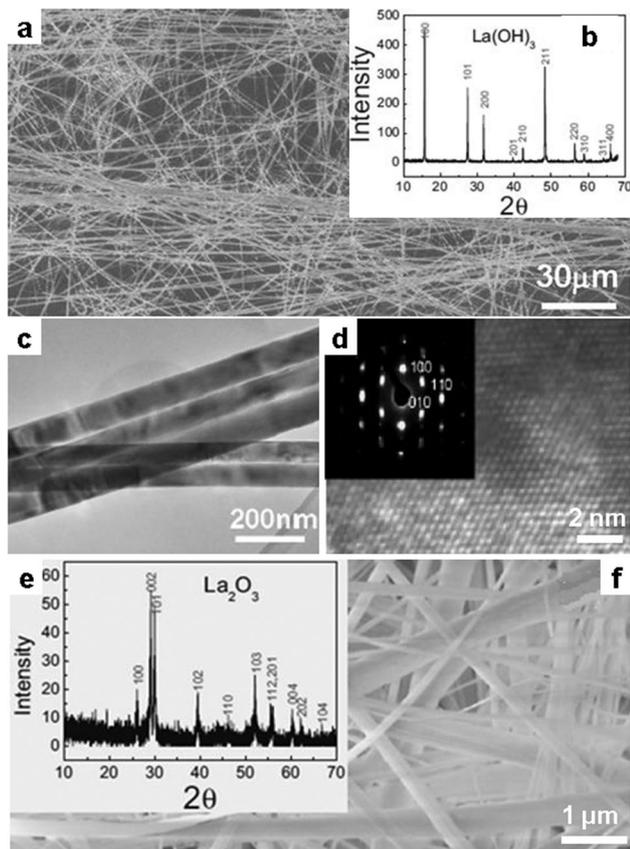
**Fig. 5**  $\text{La}(\text{OH})_3$  nanobelt produced in the melt of  $\text{NaOH}/\text{KOH}$  at  $200\text{ }^\circ\text{C}$  from  $\text{La}(\text{Ac})_3$  observed by (a) SEM image, (b) XRD pattern, (c) TEM and (d) high resolution TEM (HR-TEM) images. (e) XRD and (f) SEM image of the  $\text{La}_2\text{O}_3$  nanobelts by thermal decomposition of  $\text{La}(\text{OH})_3$  at  $690\text{ }^\circ\text{C}$ . (Reprinted with permission from ref. 64. Copyright 2007 John Wiley and Sons.)
