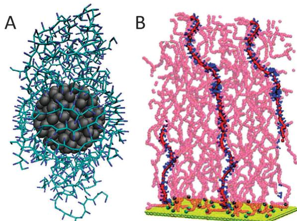
**Fig. 8** Polymeric systems. (A) Nanoparticle coated with PMMA resin<sup>278</sup> (courtesy Y. Huang). Nanoparticle is shown in grey, the polymer in blue. (B) Grafted polystyrene chains in good solvent<sup>279</sup> (courtesy G. Rossi). Support is shown in yellow, polymer backbone in red with one polymer highlighted with blue phenyl rings. Adapted with permission from ref. 278 and 279. Copyright (2012–2013) American Chemical Society.
