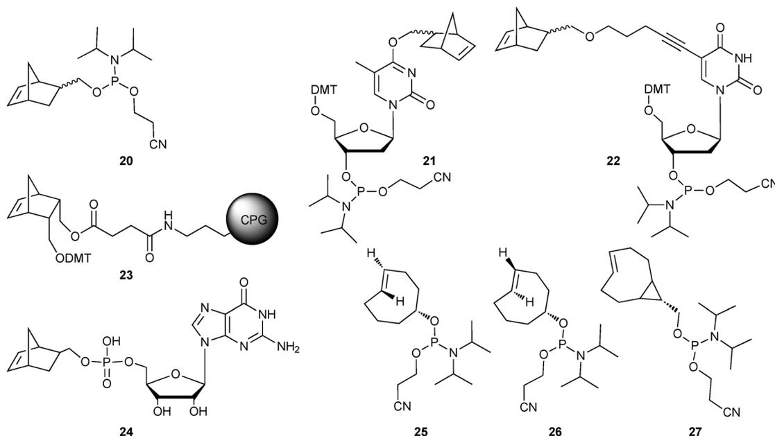
**Fig. 5** Incorporation of iEDDA dienophiles into DNA and RNA. Norbornene-containing building blocks for PCR (polymerase chain reaction) and solid phase synthesis (20–24; DMT = 4,4'-dimethoxytrityl; CPG = controlled pore glass)<sup>36,37</sup> and TCO-derivatised phosphoramidites (25–27).<sup>8</sup>
