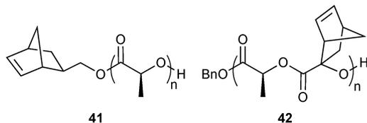
**Fig. 10** Semi-telechelic (**41**) and side-chain functionalised (**42**) poly(lactides) for iEDDA post-polymerisation functionalisation.<sup>49</sup>
