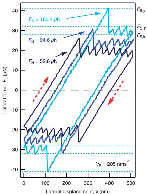
**Fig. 2** Friction loops, showing  $F_L$  as a function of  $x_s$  at a constant film thickness of  $i = 7$  and for three different values of  $F_N$ . The velocity is constant at  $v_s = 205 \text{ nm s}^{-1}$ , and the back-and-forth displacement is in the directions indicated by (red) dashed arrows. Friction features  $F_{S,y}$ ,  $F_{S,k}$ , and  $F_{S,st}$  are defined for the  $F_N = 160.4 \text{ μN}$  trace.
