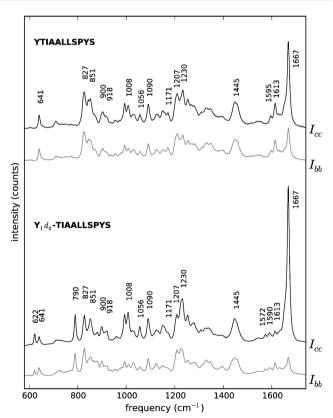
Fig. 4 Polarised Raman spectra of peptides YTIAALLSPYS (top) and Y<sub>1</sub>d<sub>4</sub>-TIAALLSPYS (bottom). Black traces: Icc spectra. Grey traces: Ibb spectra. The spectra are offset vertically for convenience. For visualisation purposes, both unlabelled YTIAALLSPYS spectra have been scaled up to approximately match the intensity of their labelled counterparts, taking the 1445 cm<sup>-1</sup> peak in the spectrum of  $Y_1d_4$ -TIAALLSPYS  $I_{cc}$  as a reference.
