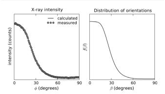
Fig. 3 Experimental and predicted intensity (left) and calculated ODF (right) for the 4.7 Å reflection of the wide angle X-ray diffraction pattern of a Y<sub>1</sub>d<sub>4</sub>-YTIAALLSPYS stalk sample
