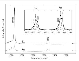
Fig. 5 Polarised Raman spectra of  $Y_1d_4$ -YTIAALLSPYS in the spectral region 1500–2800 cm $^{-1}$ . Black trace:  $I_{cc}$ . Grey trace:  $I_{bb}$ . The spectra are offset vertically for convenience. The C–D stretch vibrations appear at  $\sim 2275$  cm<sup>-1</sup>, with a higher intensity in the Ibb spectrum. Insets: C-D stretching bands at both polarisations and sub-band decomposition and fitting with Lorentzian curves.
