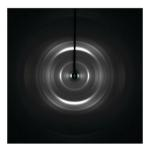
Fig. 2 Wide angle X-ray diffraction pattern of  $Y_1d_4$ -TIAALLSPYS. The stalk sample is aligned in the vertical direction. The intense meridional reflections correspond to the regular spacing between adjacent strands in the fibril axis
