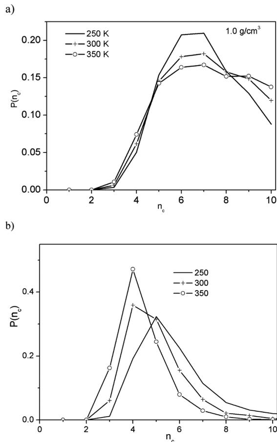
**Fig. 9** (a) Cycle size distribution in water as a function of temperature. (b) Cycle size distribution of the low density patch (neighbouring hydrogen bond number ( $k$ ) is 4).
