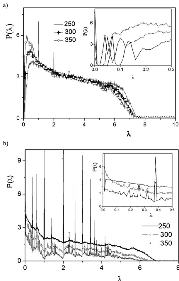
**Fig. 10** (a) Spectral density of Laplace matrix in water at different temperatures (in K). The inset shows a section of the same spectra at small eigenvalues. (b) Spectral density of Laplace matrix of water for the low density patches at different temperatures (in K).
