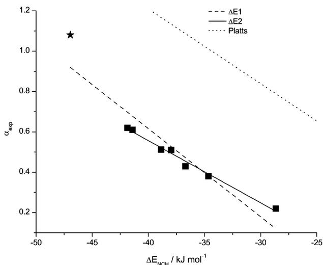
**Fig. 6** Data points and correlation functions  $\Delta E1$  and  $\Delta E2$  for  $\Delta E(\text{NCH})$  with the H-bond acidity  $\alpha$ , together with the function established for molecular solvents. Problematic data points are starred.
