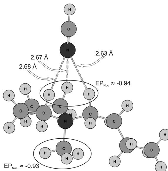
**Fig. 5** Bonding pattern in the  $[\text{C}_4\text{C}_1\text{py}]^+\cdots\text{NCH}$  complex.
