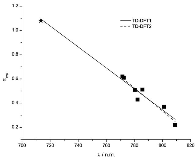
Fig. 8 Data points and correlation functions TD-DFT1 and TD-DFT2 for  $\lambda(\text{RD})$  with H-bond acidity  $\alpha$ . The star indicates that the second excitation wavelength is more appropriate and has been used.
