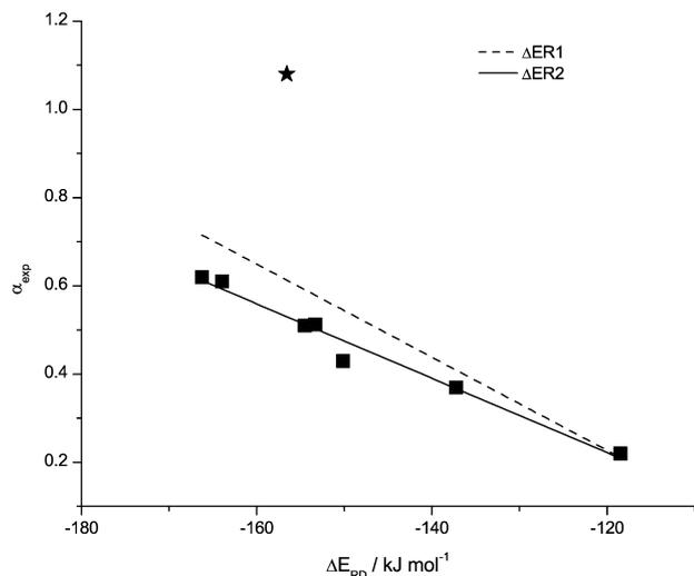
**Fig. 9** Data points and correlation functions for ER1 and ER2 for  $\Delta E(\text{RD})$  with the H-bond acidity  $\alpha$ . Star indicates the outlier  $[(\text{HOC}_2)_3\text{C}_1\text{N}]^+$  cation.
